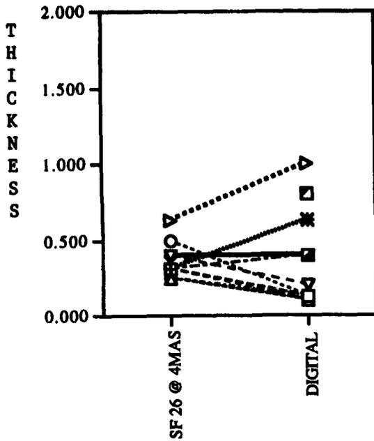
Chart: 4 mAs, screen film and digital. The screen film (SF) system performs better for some objects sizes and less well for others when compared to the digital system. The digital system system shows one object (0.2 mm) that is smaller than those seen with the screen film system.
