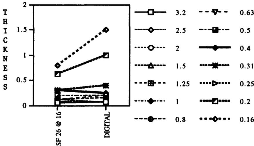
Chart: at 16 mAs, the screen film system shows thinner objects for all object sizes than does the digital system. At 16 mAs, both systems showed the 0.16 mm diameter object. This object could not be seen with 4 or 6 mAs.
