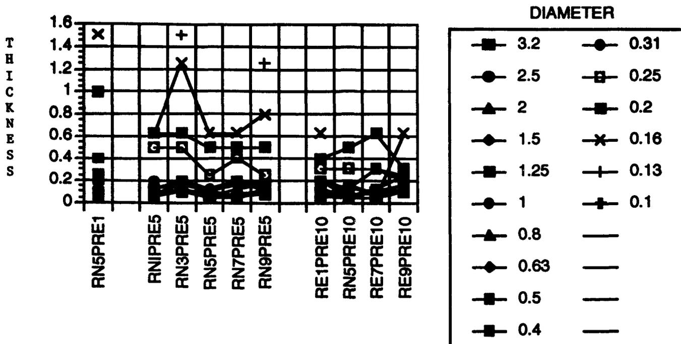
This graph demonstrates that with increasing spatial frequency filtering intensity (demonstrated as increased RE factors), objects could be detected at thinner diameters. However, at the highest intensity (RE = 10), the smallest objects (0.13 mm) could not be detected, most likely due to the exaggeration of noise which simulated small calcium like densities.
