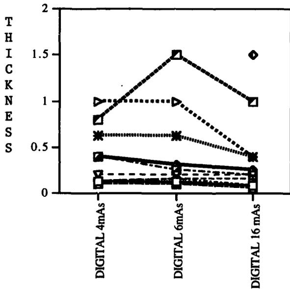
This chart shows for the digital system, that increased exposure between 4 to 6 mAs had little effect on detection. Increases to 16 mAs showed improved resolution with a smaller object seen and with thinner objects seen.
