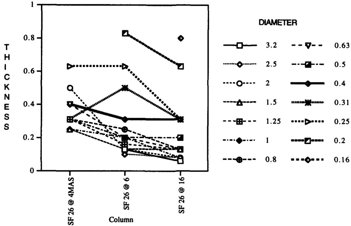
This chart demonstrates that with increasing exposures in the screen film system, the disks on the CDMAM phantom could be seen both thinner and with smaller diameters as exposure increased from 4 to 6 to 16 mAs.
