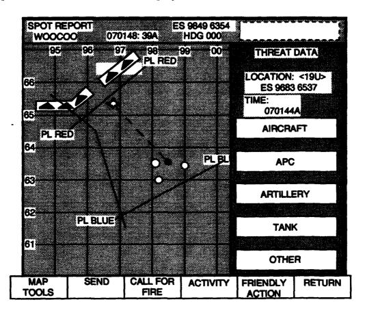
The black dot represents the location of the tank in which you are riding and on whose IVIS screen you are looking. Its own location, as determined by its on-board, inertial, position navigation system (POSNAV), is displayed in the upper box on the display (ES 9849 6354). The three open circles are the other tanks in the platoon whose positions are digitally reported over the platoon radio net at a prescribed interval or whenever they move a specific distance.
