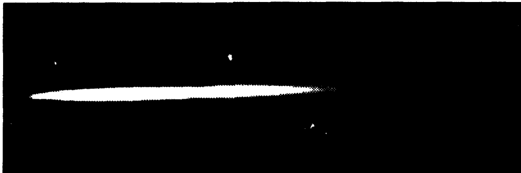
Figure 10. Averaged images of SF 6 /CO 2 and SF 6 /N 2 spray at Tr = 0.95 and Pr = 1.0
