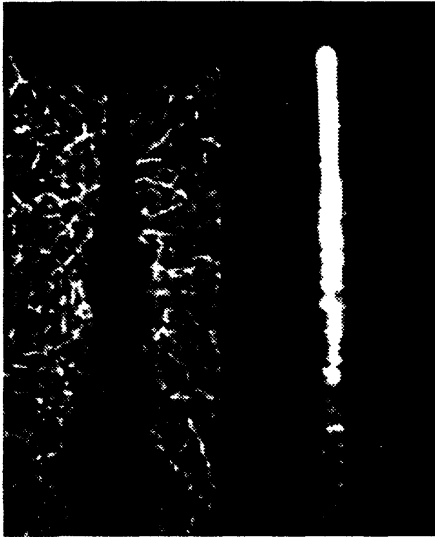
Figure 12. Instantaneous Image of SF 6 /N 2 Sprays at Pr = 1.0.
