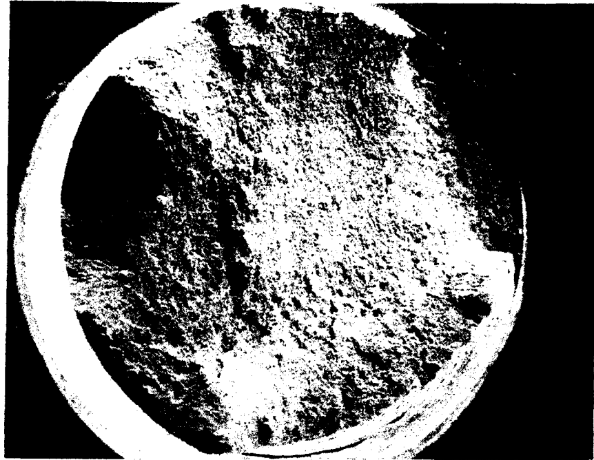
Figure 20a Low magnification scanning electron micrograph of the HY-100 parent metal showing the embrittled behavior observed in failures contained in Region III of Figure 6.
