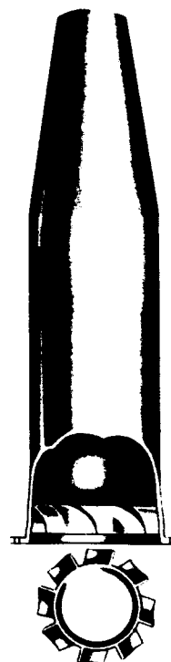
Fig. 2.4—Multiclone Tube Showing Inlet Vanes (Western Precipitation Corp.)
