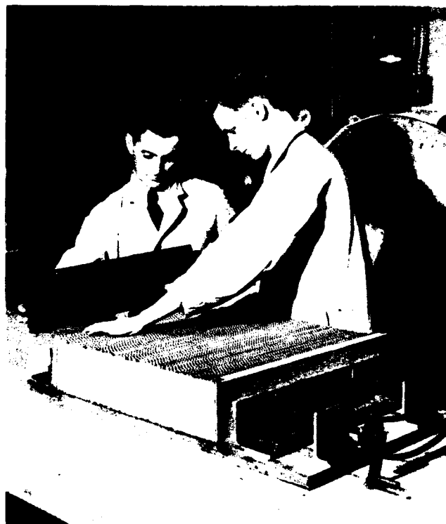
Fig. 2.34—Manufacture of Cellulose-Asbestos Paper - Note the corrugated paper spacers between the pleats of the filter medium. (A. D. Little, Inc.)
