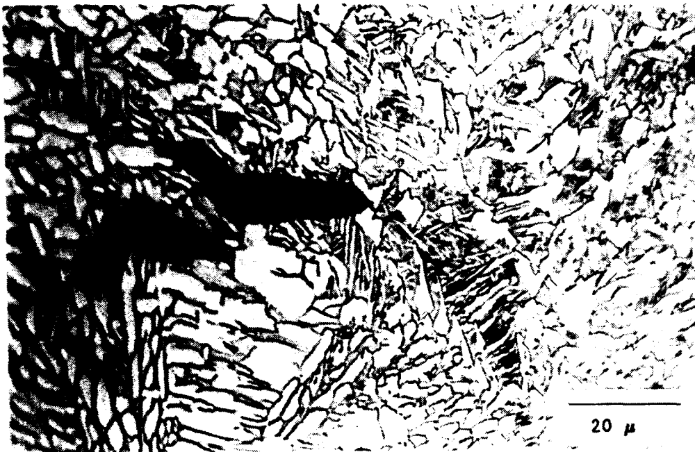
Figure. 16. Longitudinal cross section of a failed tensile specimen as-ROC'ed and tested at 427°C (800°F), showing (a) flat transverse fracture surface, with multiple transverse cracks in the longitudinal direction on the specimen surface and microvoids nucleated within the specimen, and (b) bridging of two cracks at the same horizontal plane.
