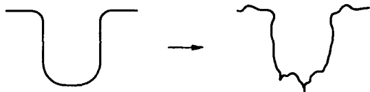
Figure 4 Worst case impression of a blunt weak flaw with "aging pits" and sharp flaws.
