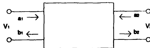
Figure 1: Two - Port Network
