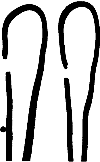
Figure 6 Failed copper tail wires of an aerial clamp
