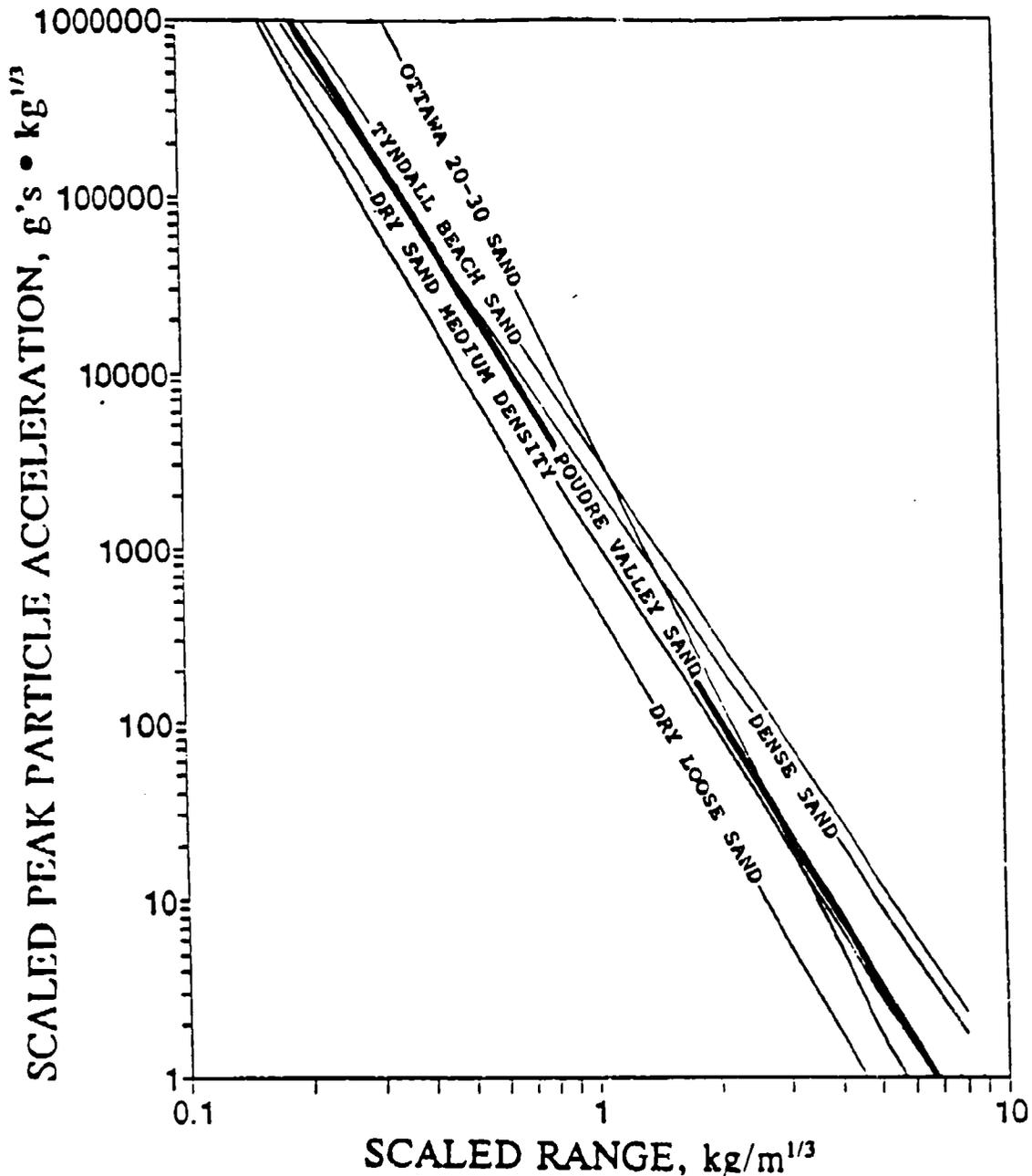
note: equations for average scaled peak particle acceleration are used to plot curves for Poudre Valley, Tyndall Beach and Ottawa 20-30 sands (see Section V.B.4 for development of equations).
