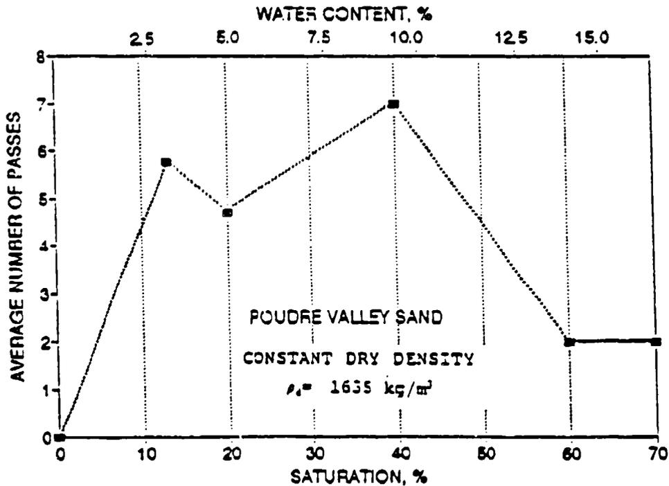
Figure 4.3 Compactive Effort (Number of Passes with Vibratory Compactor) versus Percent Saturation to Reach a Constant Dry Density of  $1635 \text{ kg/m}^3$  for Poudre Valley Sand.
