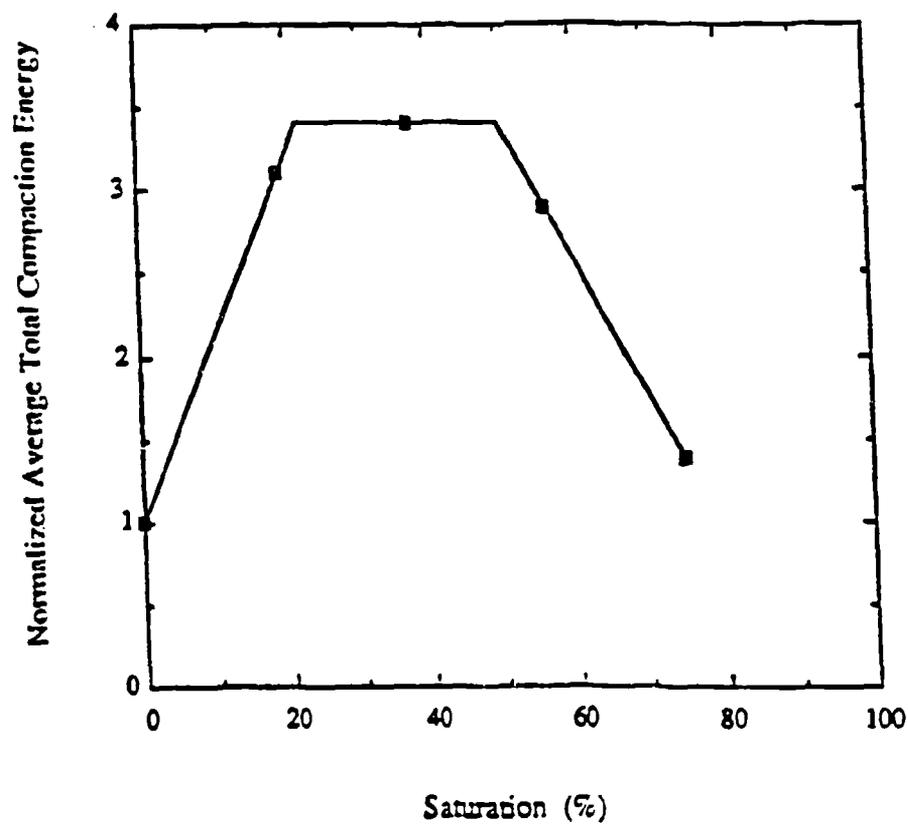
Figure 2.10 Normalized Average Total Compactive Energy for Ottawa 20-30 Sand Compacted to a Dry Density of  $1715 \text{ kg/m}^3$  (Veyera and Fitzpatrick, 1990).
