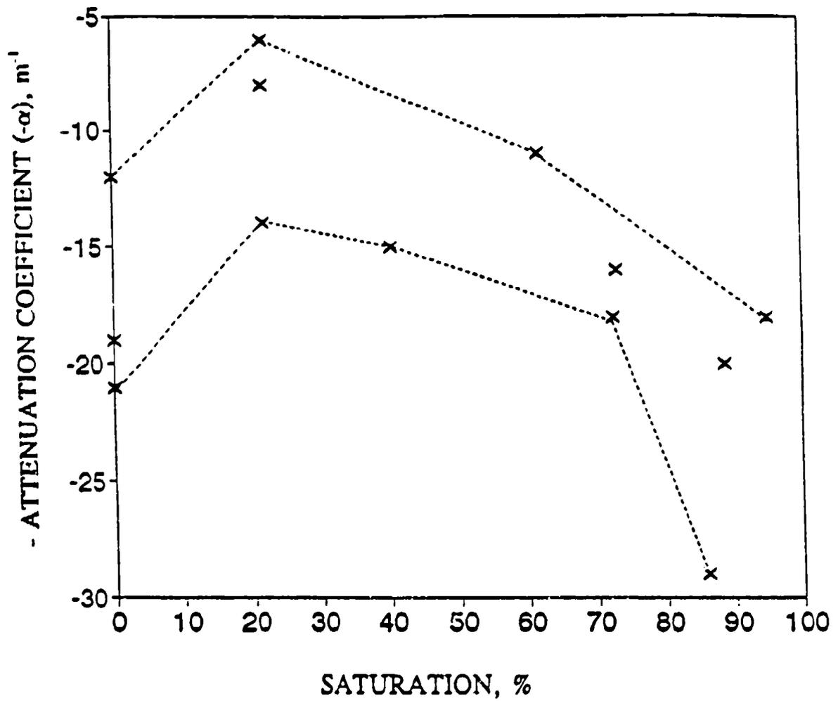
Figure 2.6 Attenuation Coefficient versus Percent Saturation for 50/80 Silica Sand (Plotted from Test Results from Charlie et al., 1990a).
