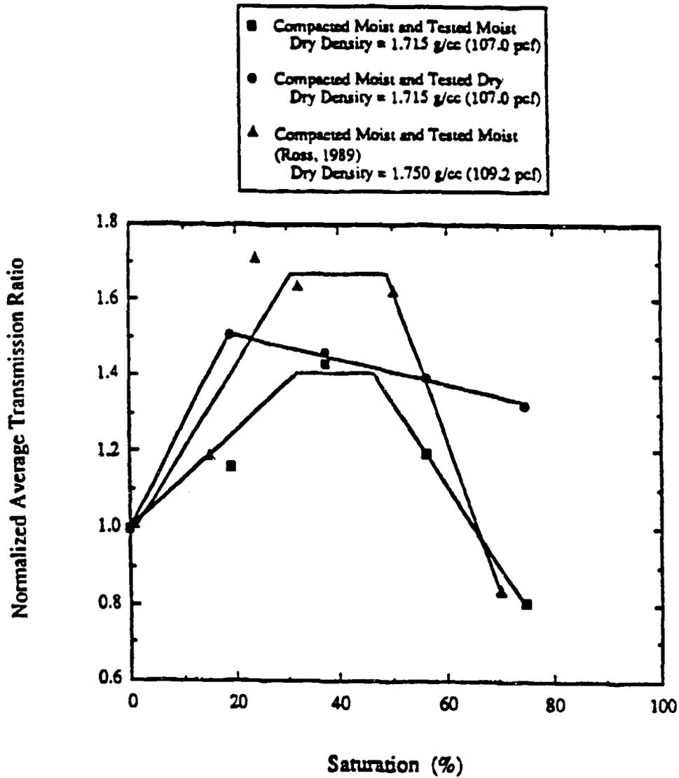
Figure 2.9 Normalized Average Transmission Ratio as a Function of Saturation for Ottawa 20-30 Sand (Veyera and Fitzpatrick, 1990).
