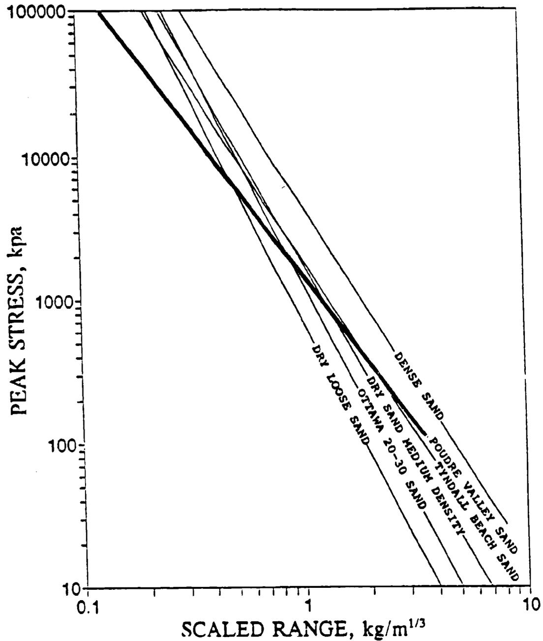
note: equations for average peak stress are used to plot curves for Poudre Valley, Tyndall Beach and Ottawa 20-30 sands (see Section V.B.4 for development of equations).
