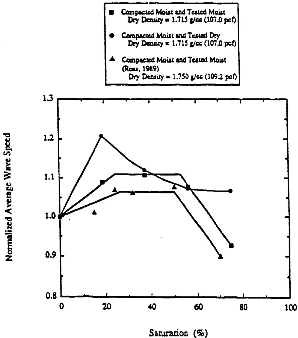
Figure 2.8 Normalized Average Wave Speed as a Function of Saturation for Ottawa 20-30 Sand (Veyera and Fitzpatrick, 1990).
