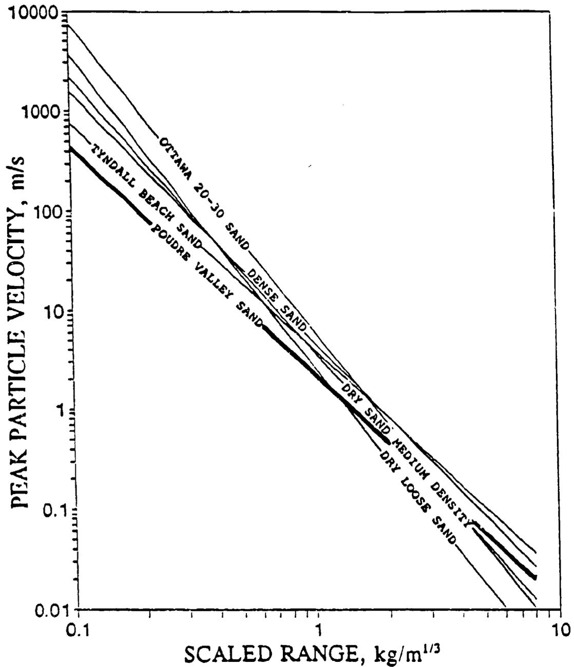
note: equations for average peak particle velocity are used to plot curves for Poudre Valley, Tyndall Beach and Ottawa 20-30 Sands (see Section V.B.4 for development of equations).
