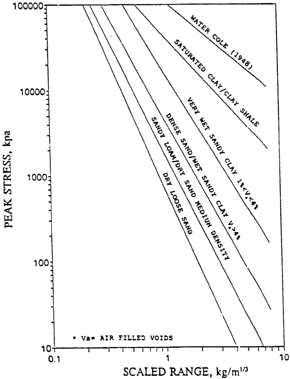
Figure 2.4 Peak Stress versus Scaled Range from Explosions in Varying Soil Types (Plotted using Drake and Little's Equations and Design Coefficients, 1983 and Cole's Equation for Water, 1948).
