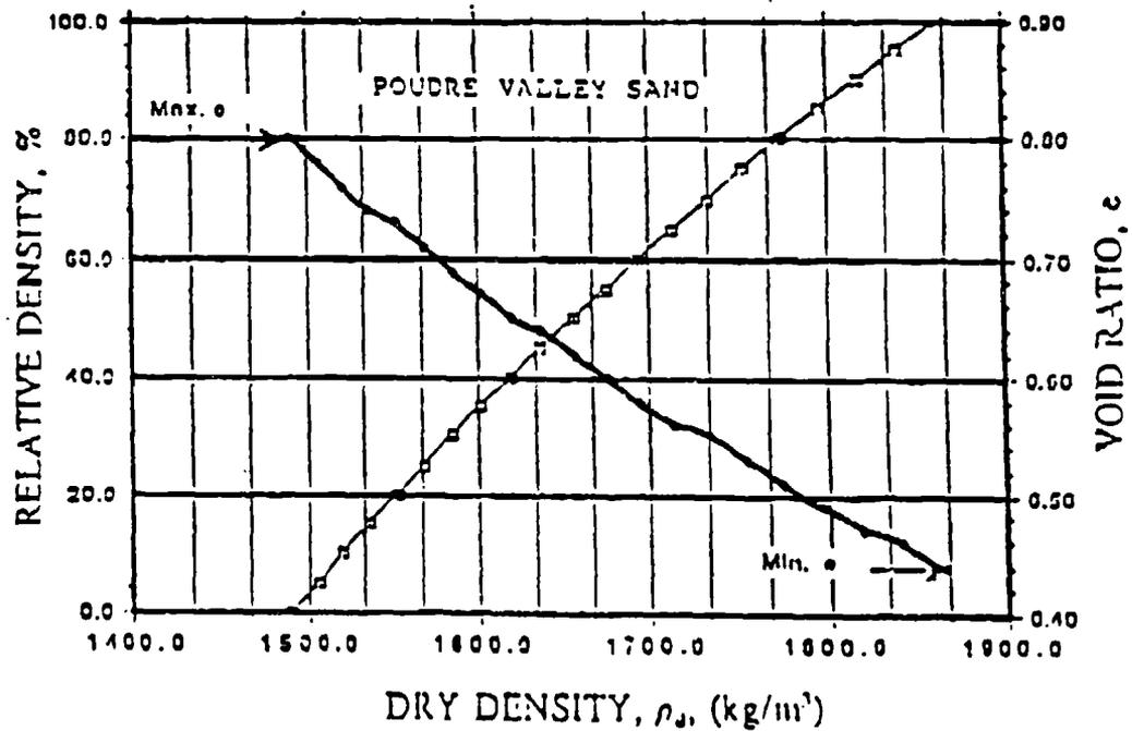
Figure 4.6 Relative Density and Void Ratio versus Dry Density for Poudre Valley Sand (Bureau of Reclamation Soil Mechanics Laboratory--Denver, Colorado).
