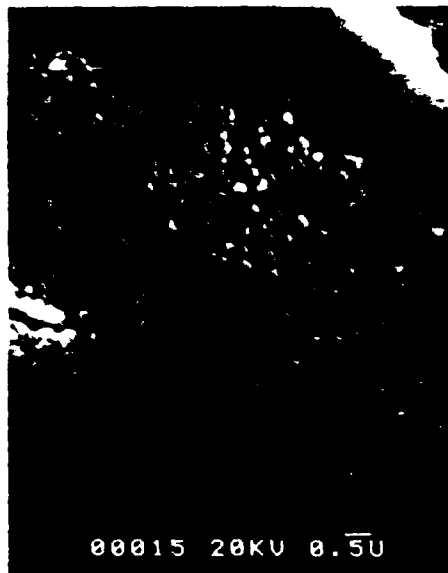
Fig. 11. SEM micrograph of a sample containing 3 mol% \text{Y}_2\text{O}_3 subjected to the following treatments: (1) sample sintered at 1450°C followed by annealing at 2100°C for 15 min and (2) surface ground and heated at 1450°C for 30 min. Note that the original grain size is ~100 \mu\text{m} (Fig. 3(c)), while the recrystallized grains have a size less than 0.5 \mu\text{m} .
