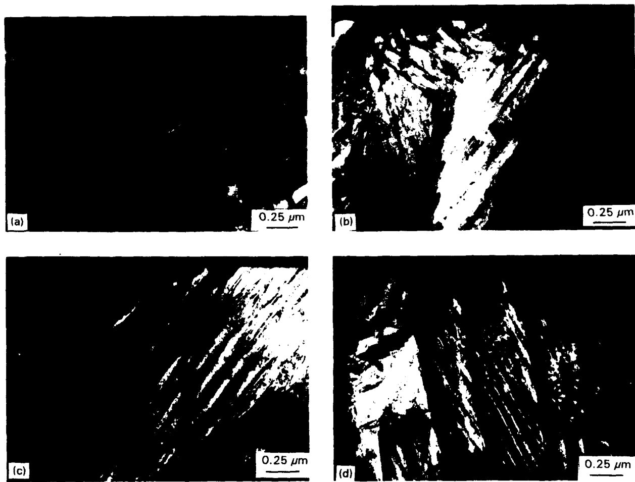
Figure 2 TEM micrographs of t' -ZrO 2 (3 mol % Ln 2 O 3 ) annealed at 2200 °C in Ar and reoxidized at 1000 °C. Note the domains in grains oriented along the [110] zone axis. (a) Ln = Dy, (b) Ln = Y, (c) Ln = Er, and (d) Ln = Yb.
