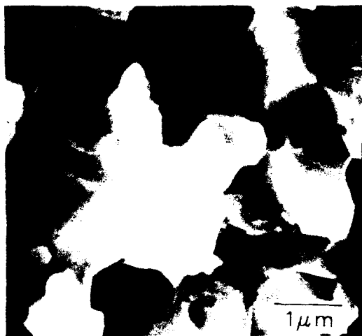
Fig. 3. SEM micrograph of fracture surface of Ce-TZP/15 vol% \text{Al}_2\text{O}_3 with 4.0 wt% \text{SrZrO}_3 . Platelet shape of strontium aluminate is clearly evident.
