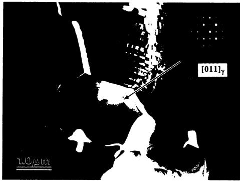
Fig. 13. Transformed  $\gamma$  grain retained in  $\beta$  grains. Large cracks generated during the  $\beta \rightarrow \gamma$  transformation (from single-phase Ca,SiO<sub>4</sub> sample sintered at 1400°C for 3 h).
