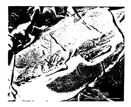
Fig. 7. SEM micrograph of MgSiO<sub>3</sub> powder calcined at 900 °C for 2 h, followed by annealing at 1400 °C for 10 h.
