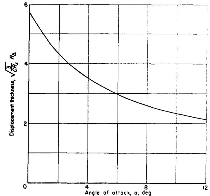
FIGURE 8.—Displacement thickness at  $\phi=0$ .  $M, 3.1$ ;  $\theta, 7.5^\circ$
