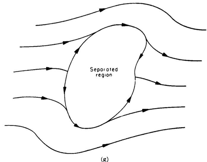
resultant shear stress at the surface and outside the separated region. The situation shown in the sketch would correspond to separation and reattachment in plane flow. If somewhere within or at the boundary of the separated region the theoretical boundary-layer solution would a priori be expected to blow up, then the vortex system within the separated region is free to roll up into a more or less vigorous system of vortices.
