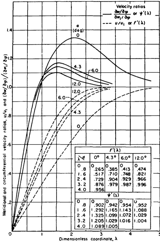
FIGURE 6.—Velocity profiles at  $\phi=0$ .  $M, 3.1$ ;  $\theta, 7.5^\circ$ .
