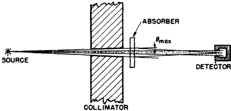
FIGURE 1. Experimental arrangement in measuring "narrow-beam" attenuation coefficients.
