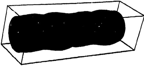
Figure 1: Schematic of two-period  $TE_{31}/TE_{11}$  beat-wave mode converter.
