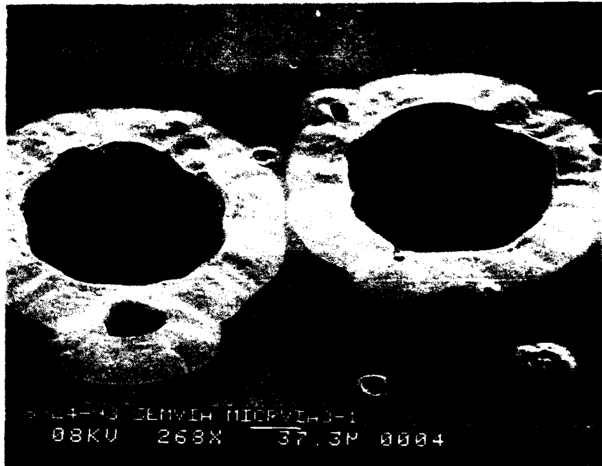
Figure 43. SEM view of silicon vias after Reactive Ion Etching (RIE) with preliminary operating parameters which caused pitting in Al mask and undercutting at via periphery. Etch depth, 95 \mu m.
