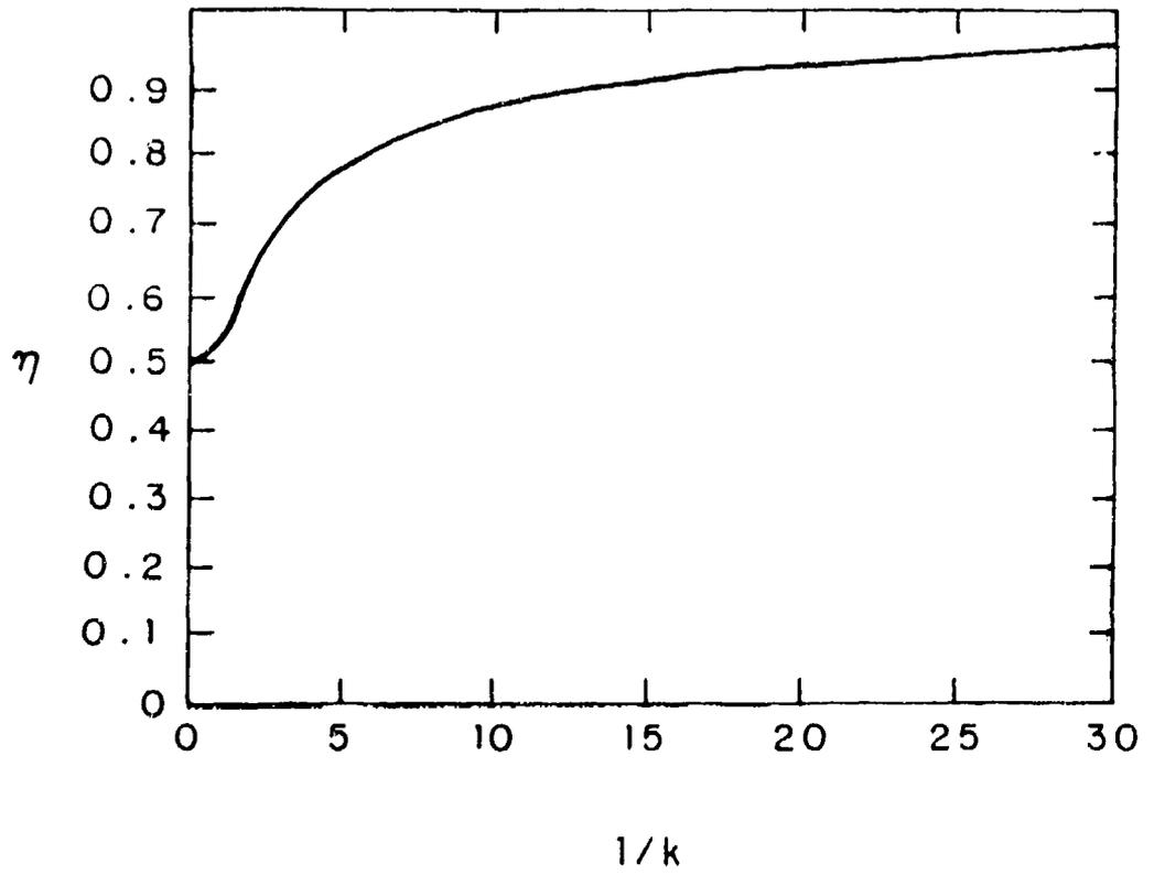
Figure (5.1) Propulsive Efficiency  $\eta$  versus  $1/k$  for a plunging airfoil
