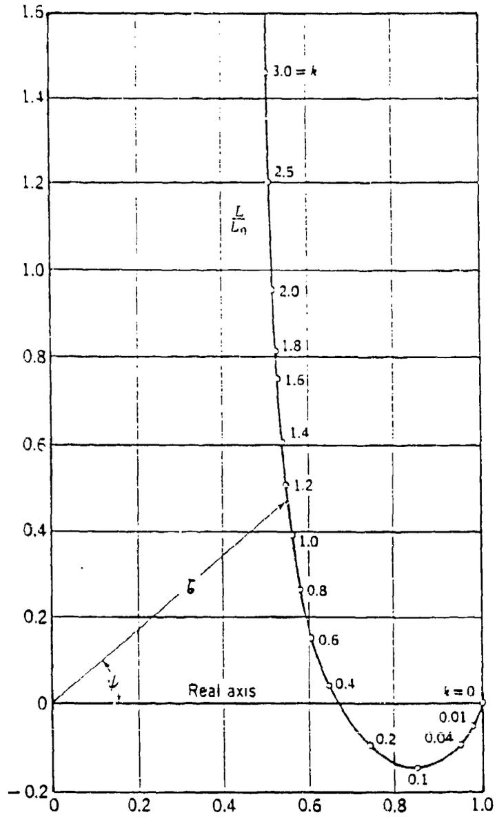
Figure (1.1)  $L/L_0$  Phase Diagram ( Imaginary vs Real ).
