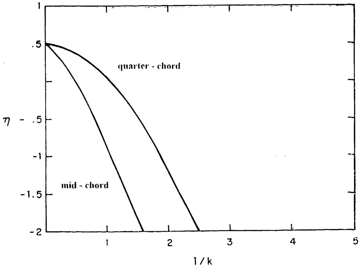
Figure (5.3) Propulsive Efficiency  $\eta$  versus  $1/k$  for an airfoil pitching about the quarter - chord point and mid - chord point
