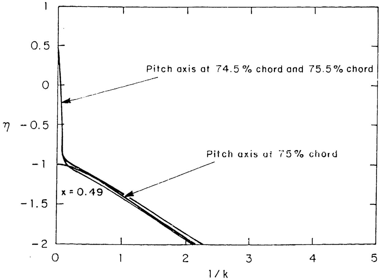
Figure (5.4) Propulsive Efficiency  $\eta$  versus  $1/k$  for an airfoil pitching about the three-quarter-chord point
