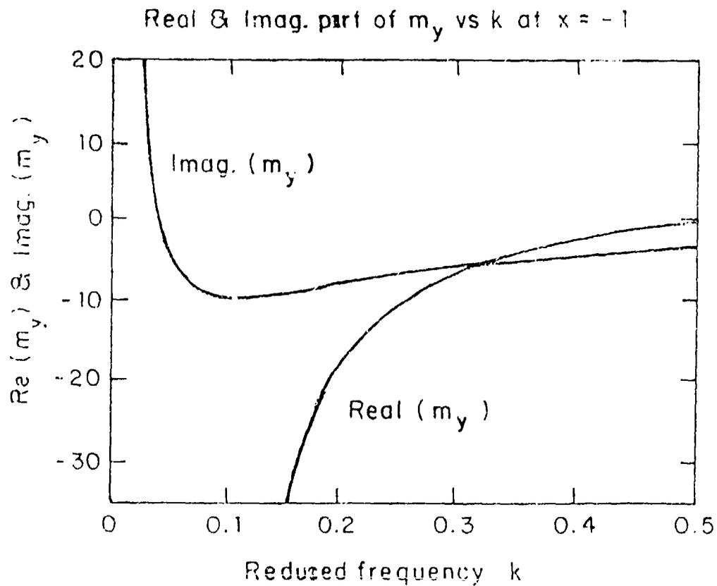
Figure (5.6) Variation with reduced frequency  $k$  of the real and imaginary parts of the non-dimensional aerodynamic moment  $m_y$  due to pitching of an airfoil about its leading edge in an incompressible flow.
