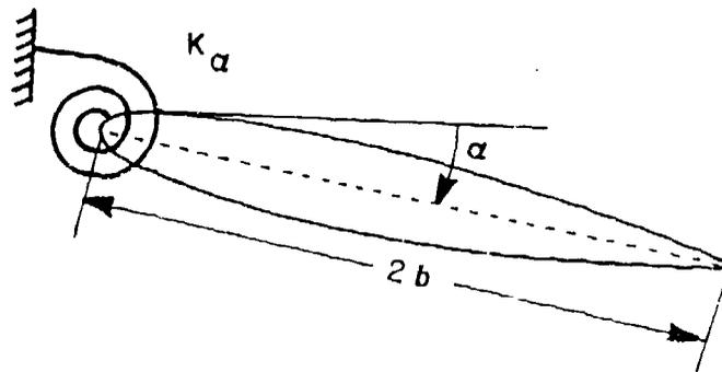
**Figure (5.5) An airfoil restrained to rotate about its leading edge in two-dimensional flow.**
