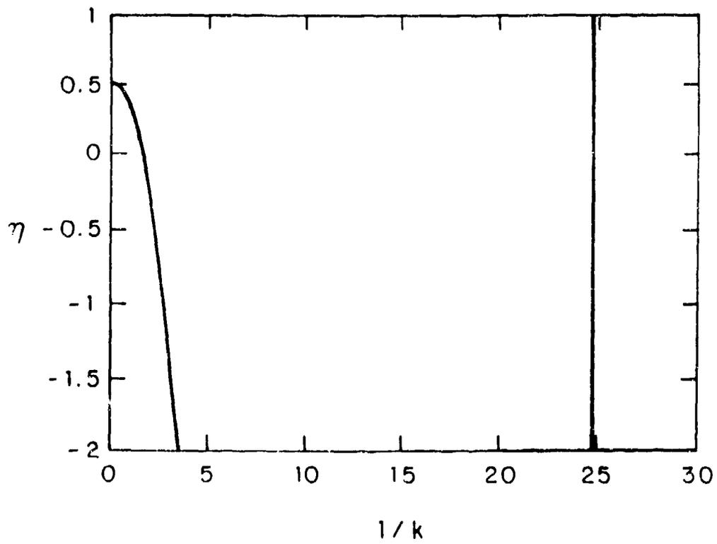
Figure (5.2) Propulsive Efficiency  $\eta$  versus  $1/k$  for an airfoil pitching about the leading edge
