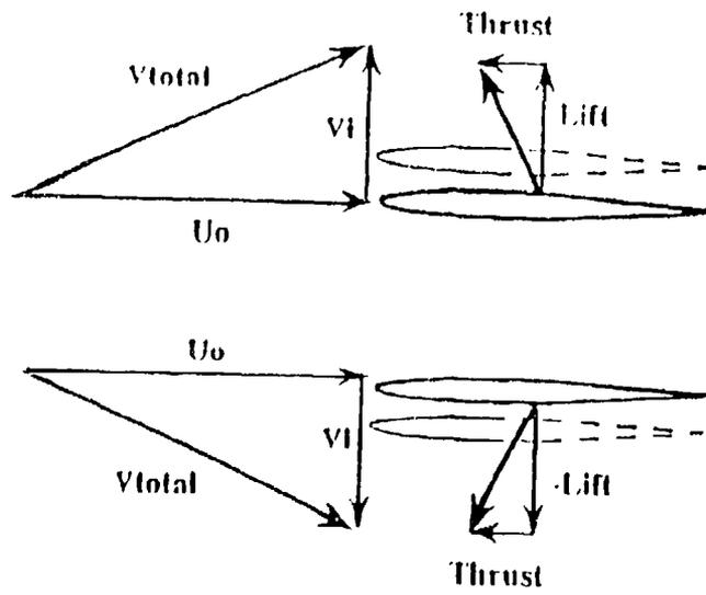
Figure (3.1) Propulsive force on plunging airfoil
