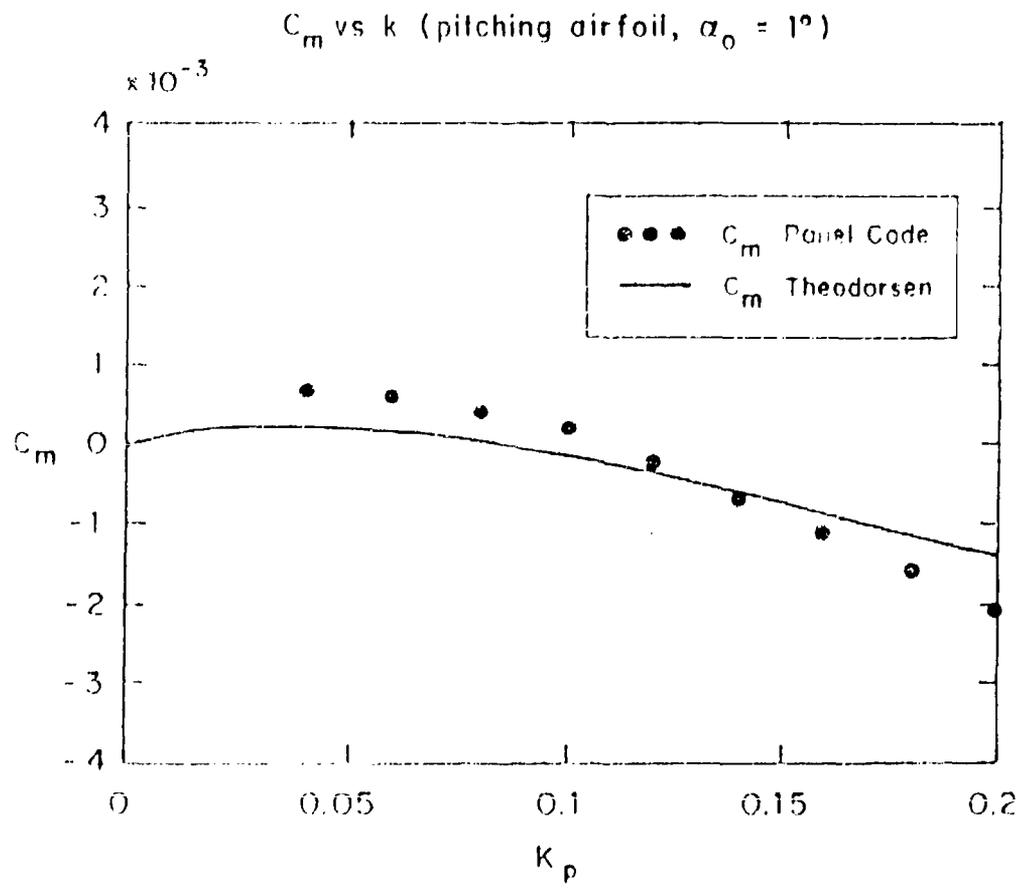
Figure (5.7) Comparison of  $C_m$  (Imag.) vs  $K_p$  for NACA0007 Oscillating in pitch about the leading edge for  $\alpha_0 = 1^\circ$  and  $N=200$  panels.
