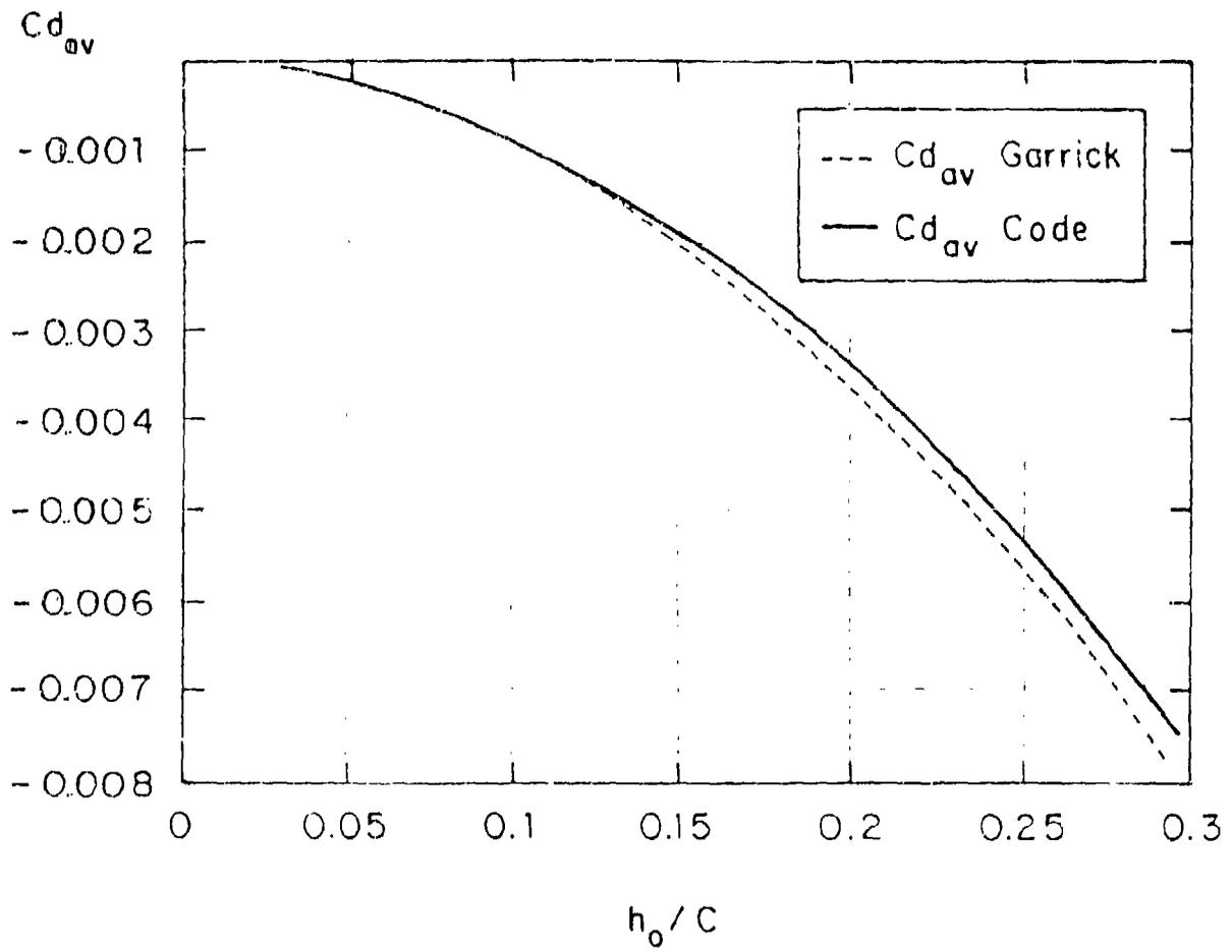
Figure (3.5) Comparison of Panel Code Results with Garrick (  $k=0.1$  )
