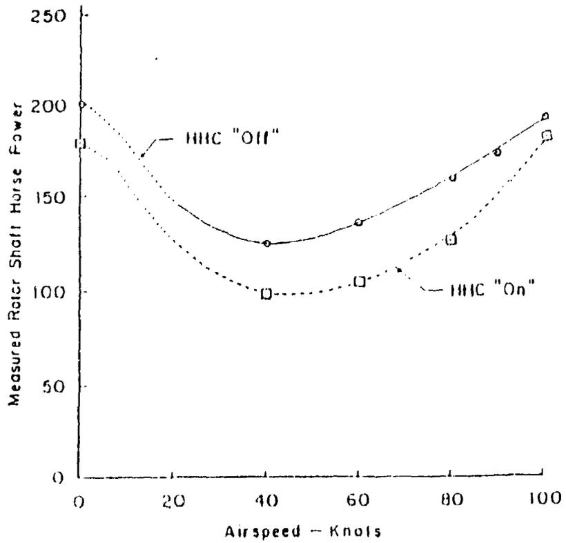
**Figure ( 1.2): Power Reduction Results from Higher Harmonic Control (HHC)
