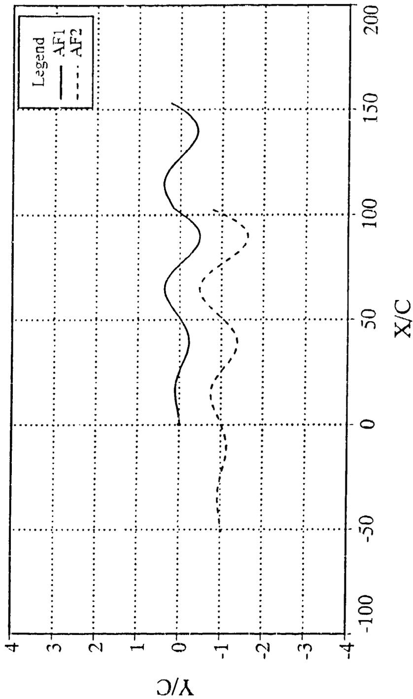
Figure (4.23) Wake pattern (pitch,  $m = 0$ ,  $h = 2$ )
