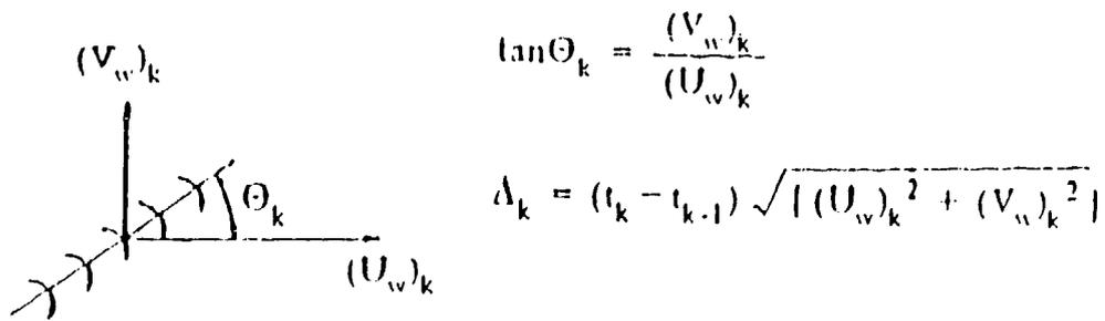
Figure (3.4) Panel Methods Representation for Unsteady Flow
