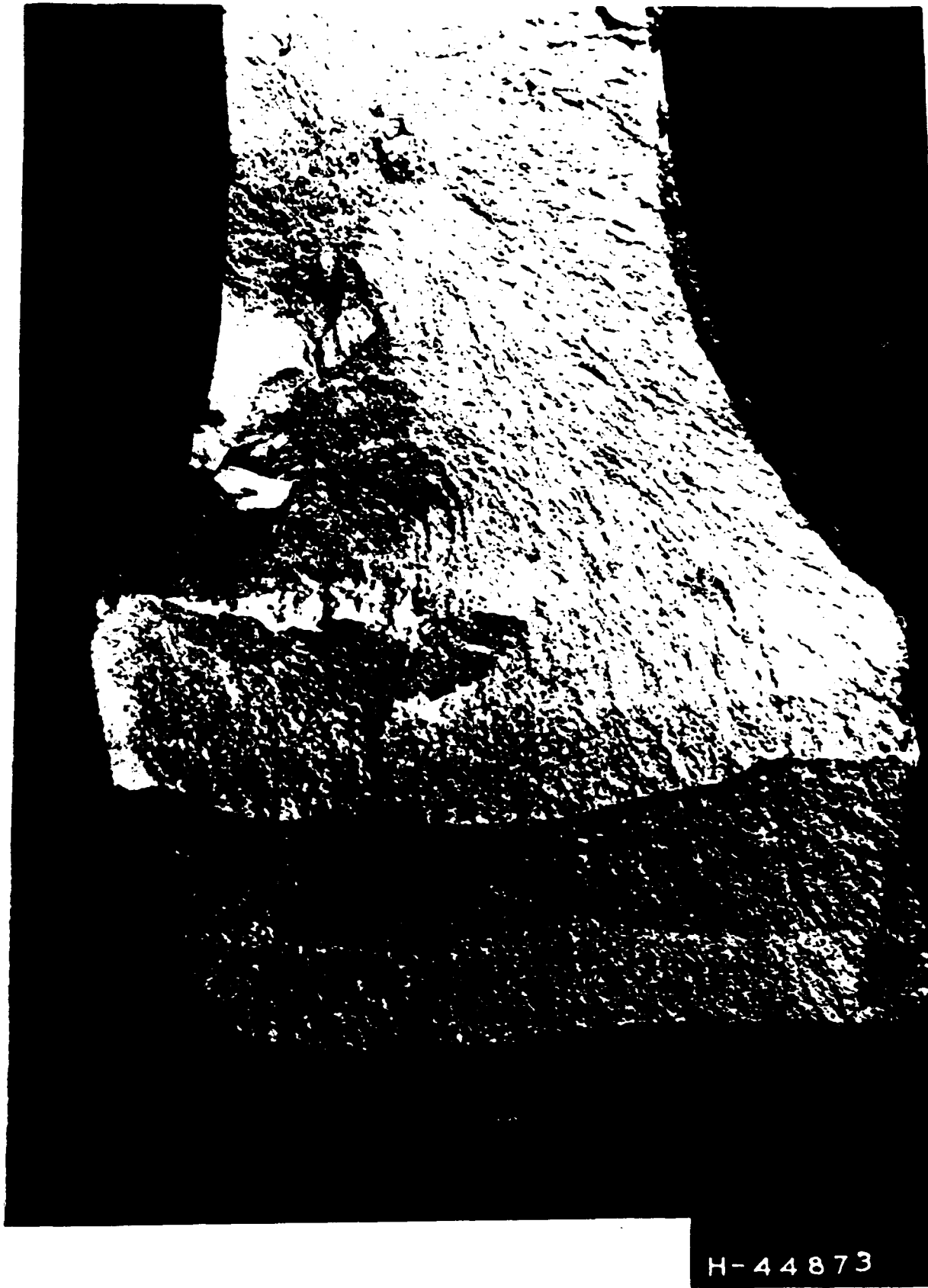
FIGURE 2 MAG: 6-1/2X SURFACE OF COMPRESSOR HUB FRACTURE SHOWING TENSILE FAILURE PROGRESSING FROM GRANULAR, BRITTLE FRACTURE AREA INDICATIVE OF CONTAMINATION.
