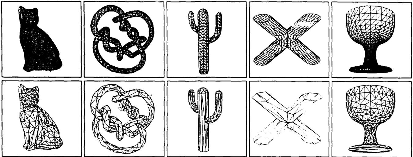
Figure 1: Examples of mesh optimization. The meshes in the top row are the initial meshes  $M_0$ ; the meshes in the bottom row are the corresponding optimized meshes. The first 3 columns are reconstructions; the last 2 columns are simplifications.
