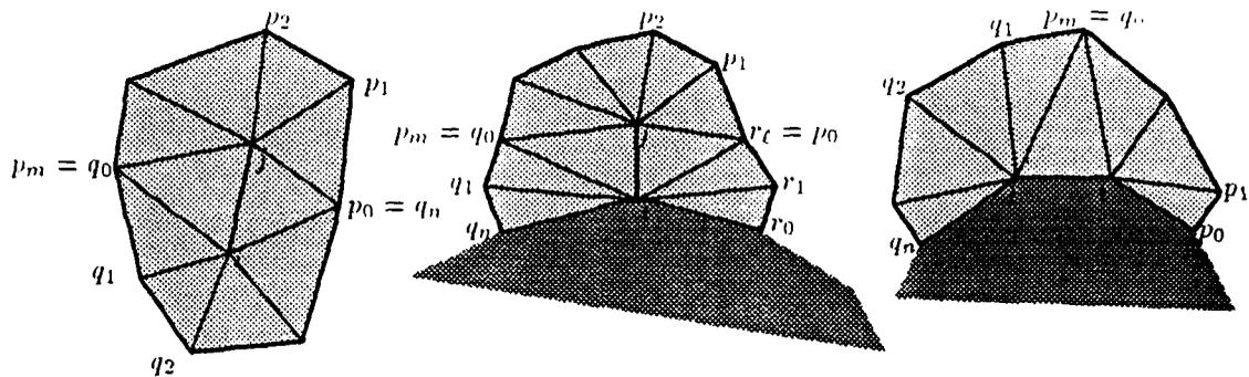
Figure 10: The sets  $N$  in the cases where: (a)  $i$  and  $j$  are both interior vertices, (b)  $i$  is a boundary vertex and  $j$  is an interior vertex, and (c)  $i$  and  $j$  are both boundary vertices.
