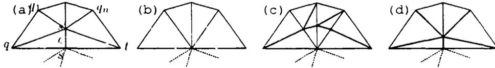
Figure 9: An edge collapse ((a)  $\Rightarrow$  (b)) can be reversed by a sequence of edge splits ((b)  $\Rightarrow$  (c)) followed by a sequence of edge collapses ((c)  $\Rightarrow$  (d)).
