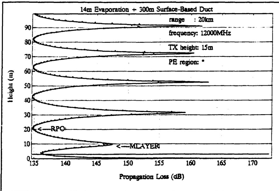
Figure D.13. Propagation loss at 20 km.
