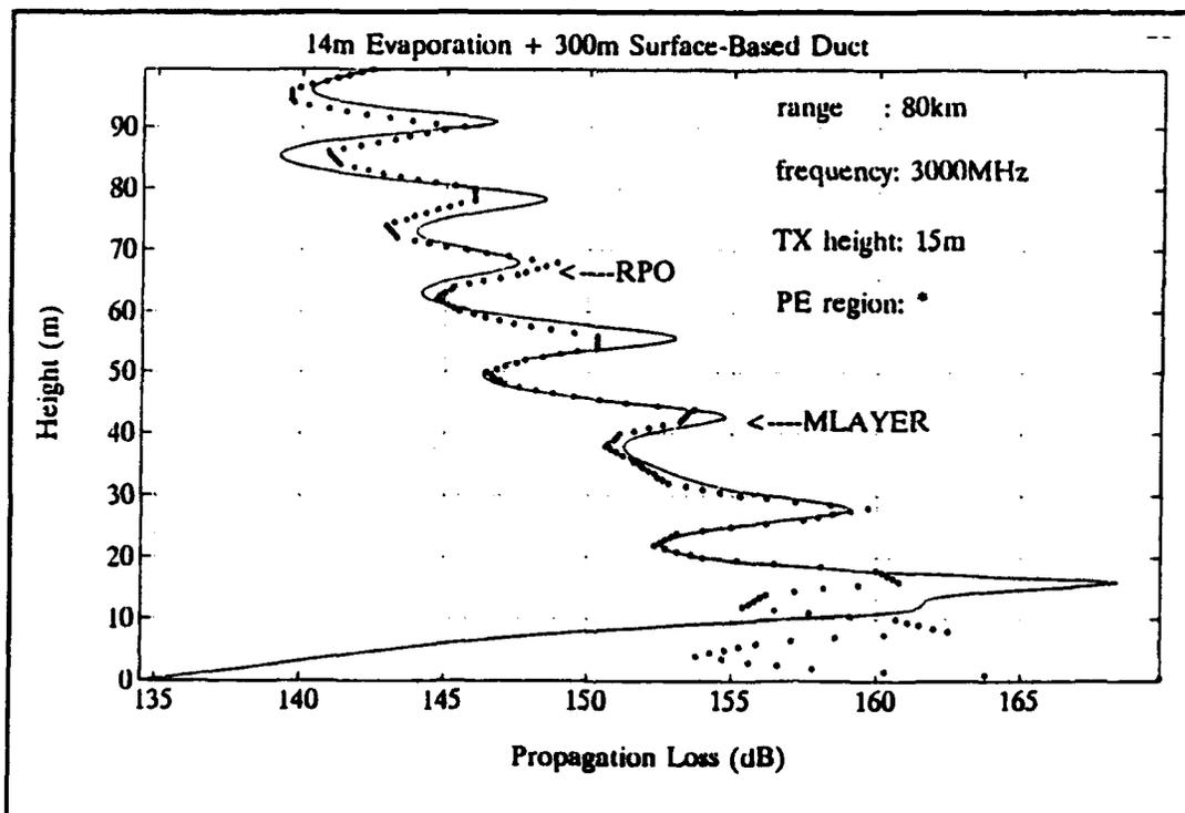
Figure D.8. Propagation loss at 80 km.
