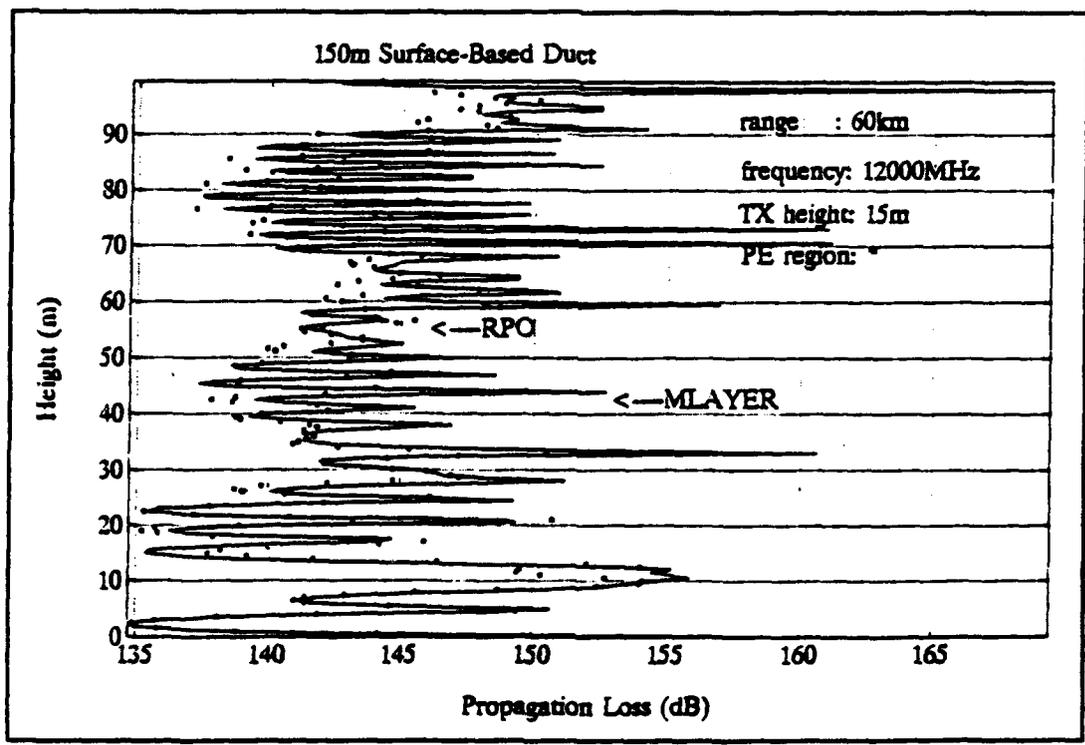
Figure E.34. Propagation loss at 60 km.
