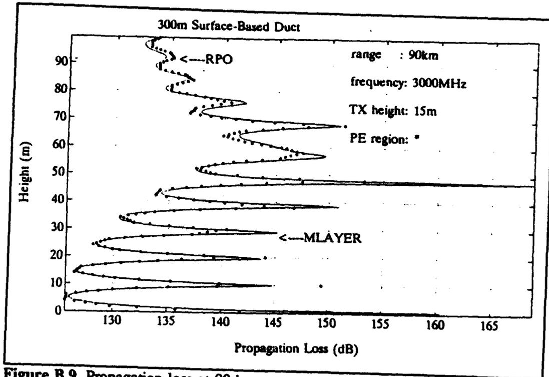
Figure B.9. Propagation loss at 90 km.
