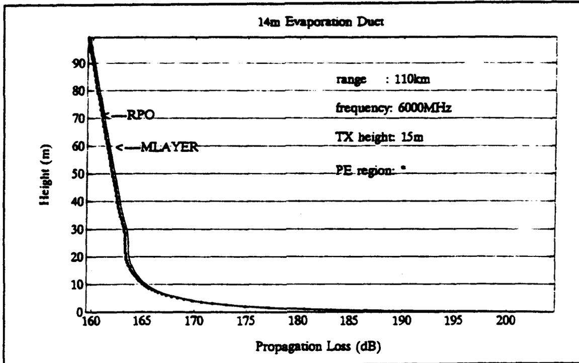
**Figure 23.** Propagation loss at 110 km.
