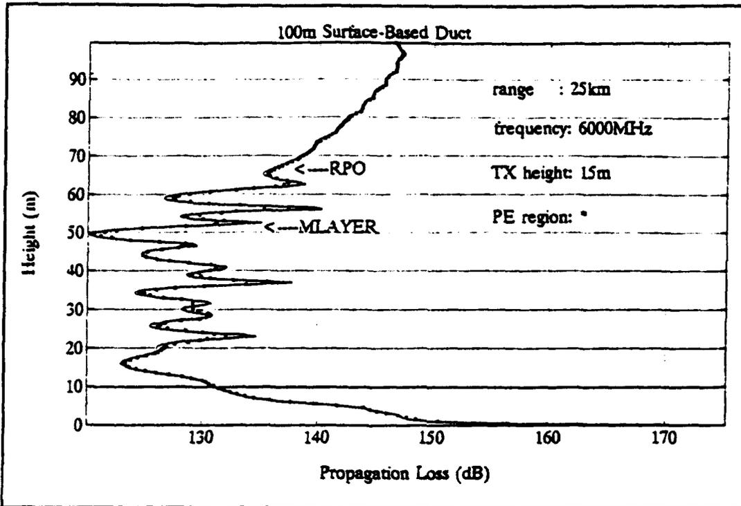
Figure F.16. Propagation loss at 25 km.
