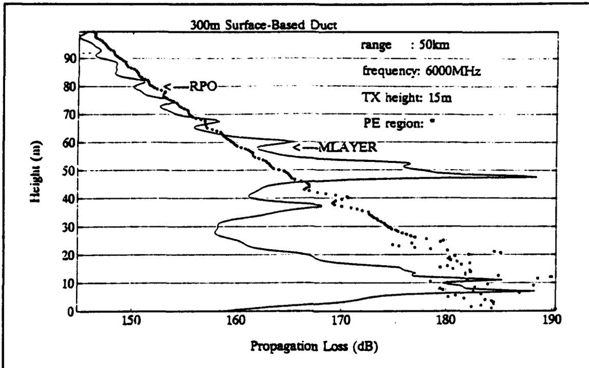
Figure 6. Propagation loss at 50 km.
