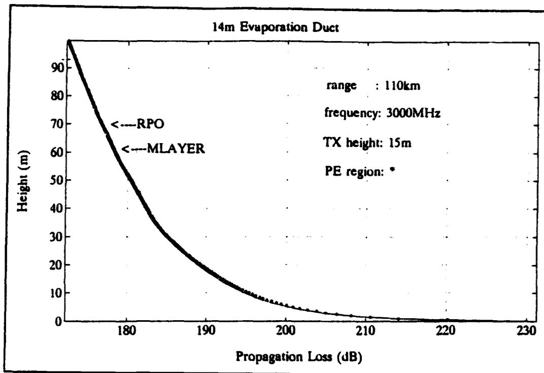
**Figure C.11. Propagation loss at 110 km.**
