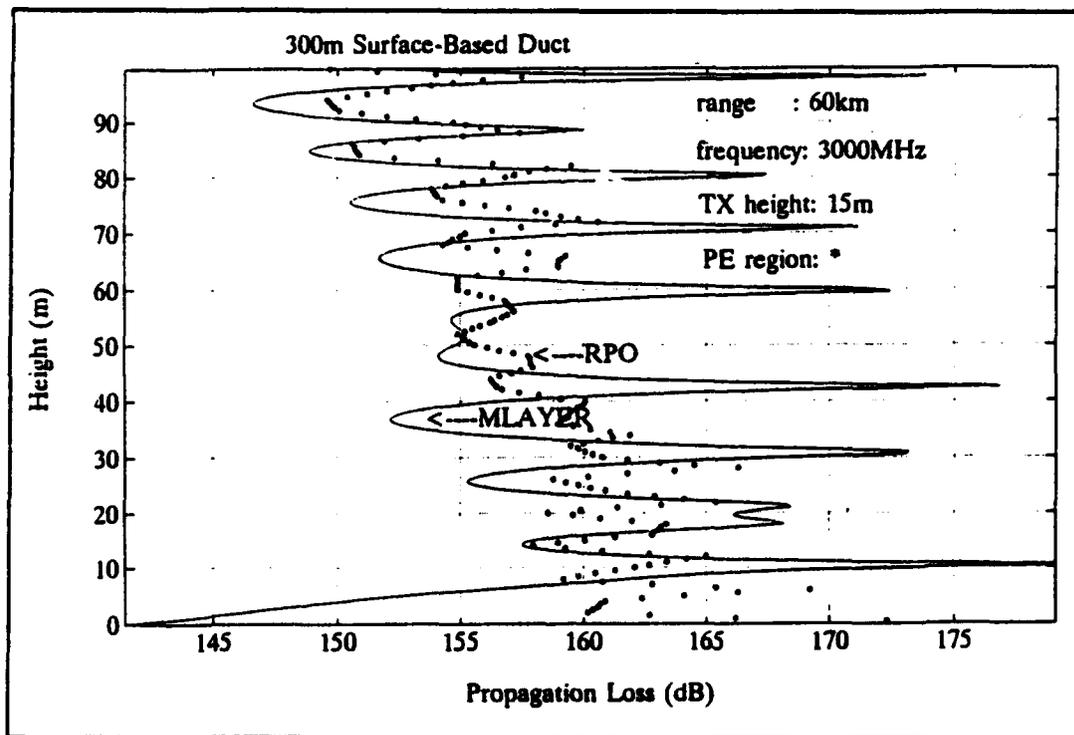
Figure B.6. Propagation loss at 60 km.
