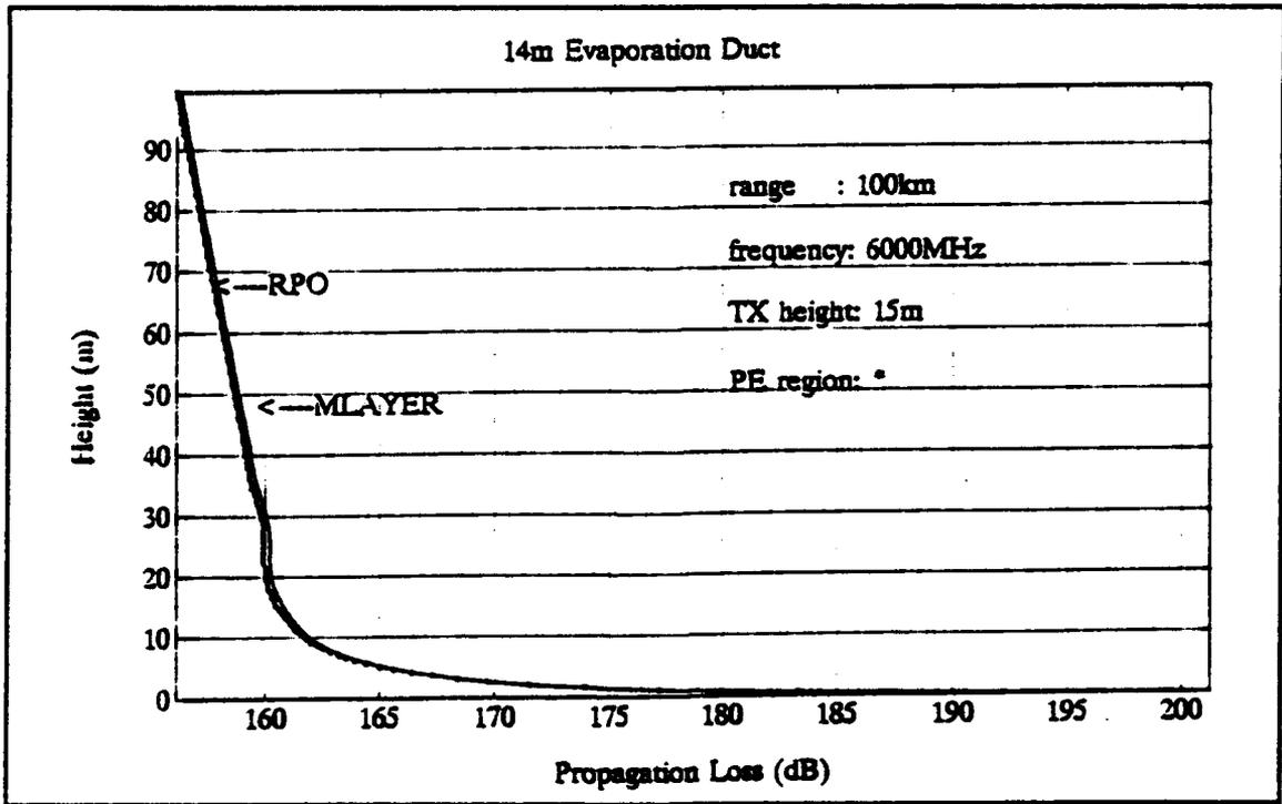
Figure 22. Propagation loss at 100 km.
