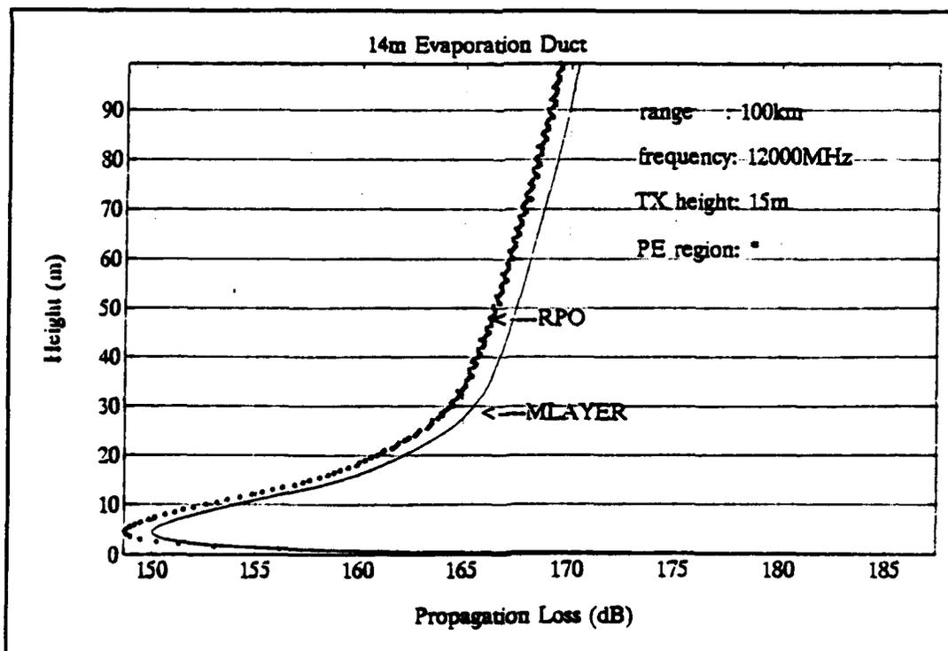
Figure C.21. Propagation loss at 100 km.
