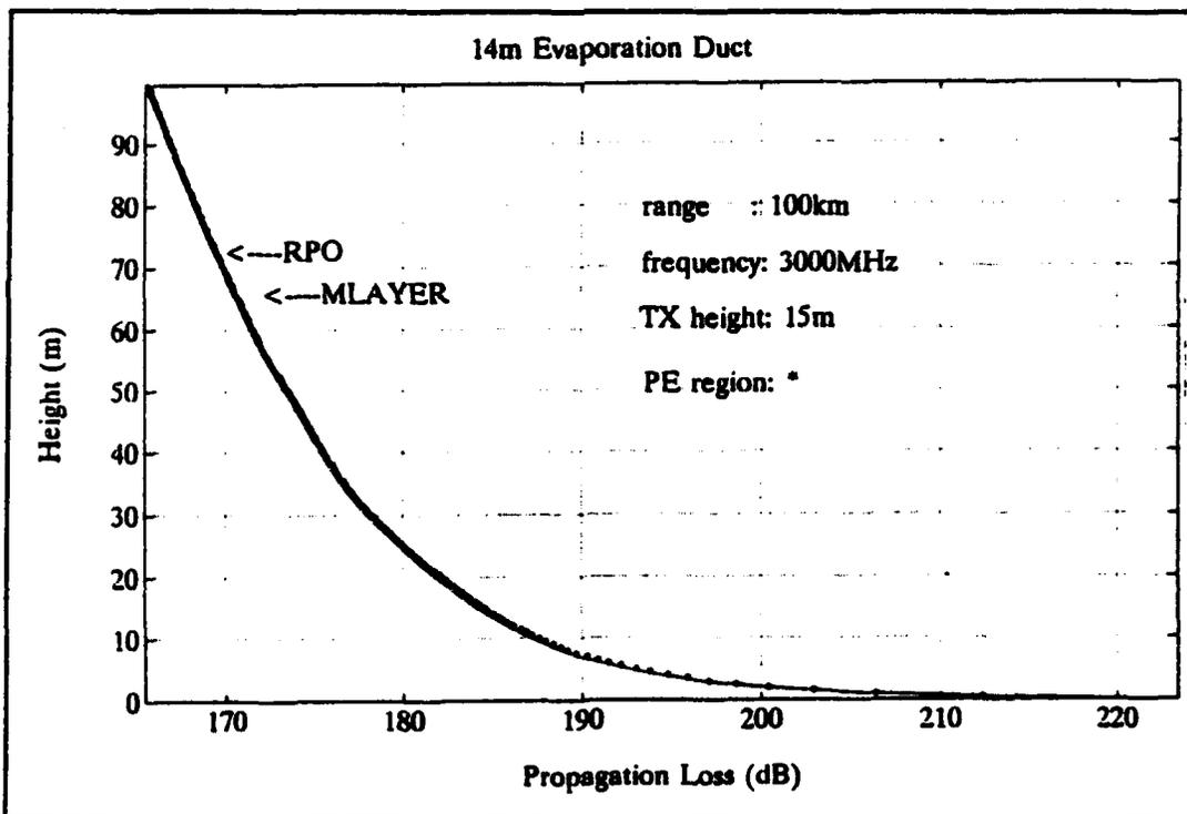
Figure C.10. Propagation loss at 100 km.
