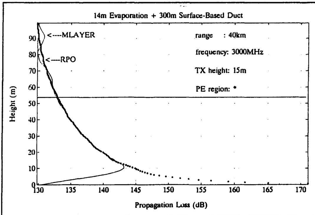
Figure D.4. Propagation loss at 40 km.
