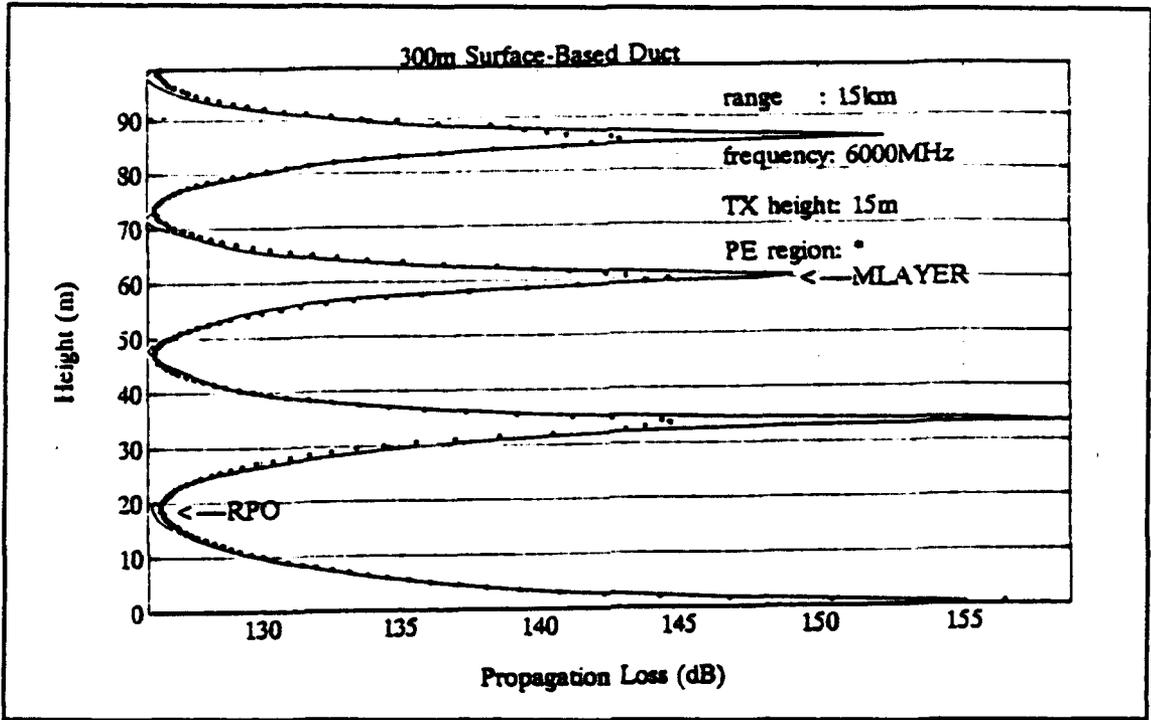
Figure 2. Propagation loss at 15 km.
