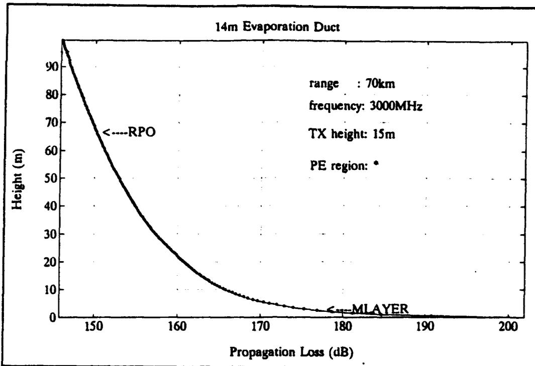
Figure C.7. Propagation loss at 70 km.
