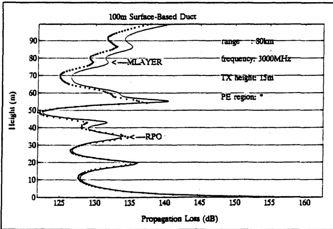
Figure F.10. Propagation loss at 80 km.
