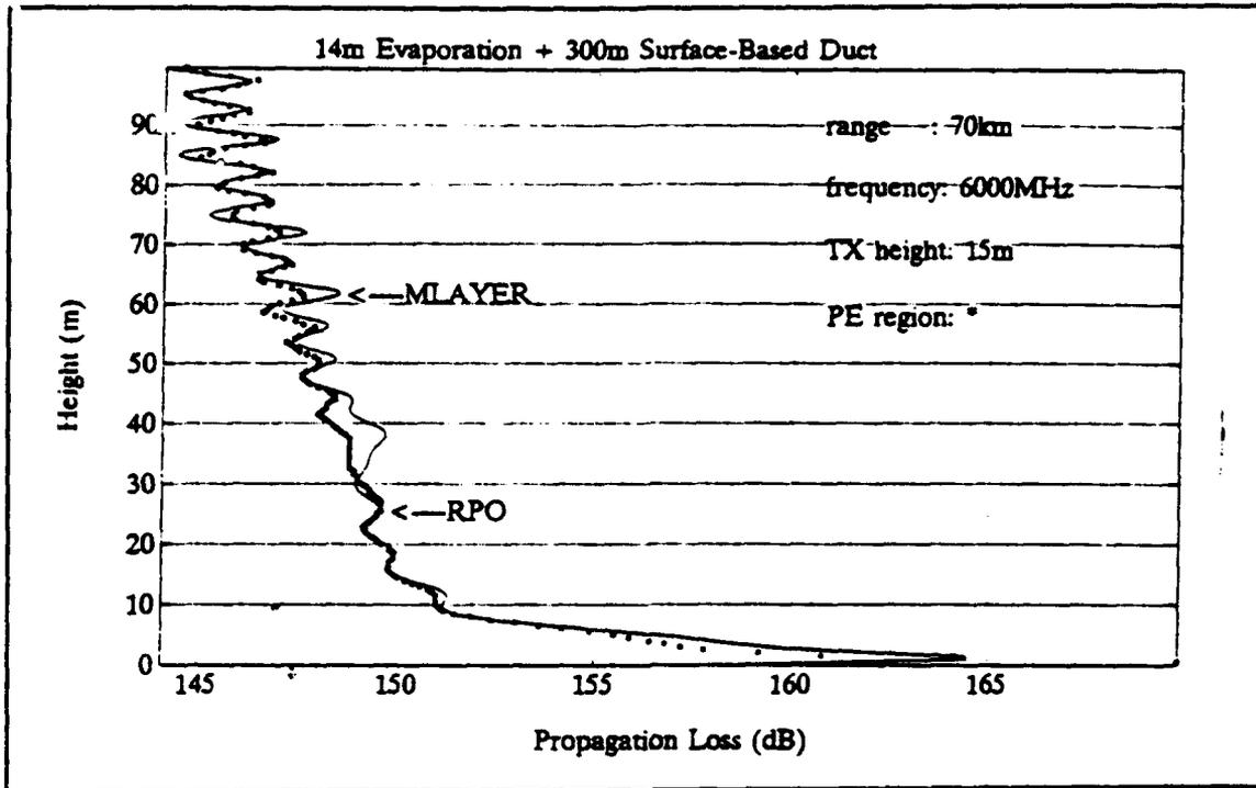
Figure 30. Propagation loss at 70 km.
