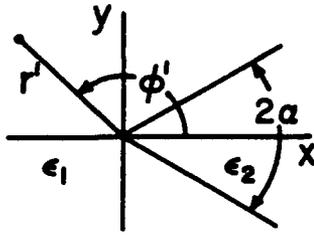
Fig. 1. Dielectric wedge and static line charge.
