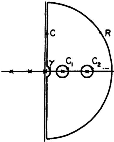
Fig. 3. Bromwich contour in the complex  $s$  plane.
