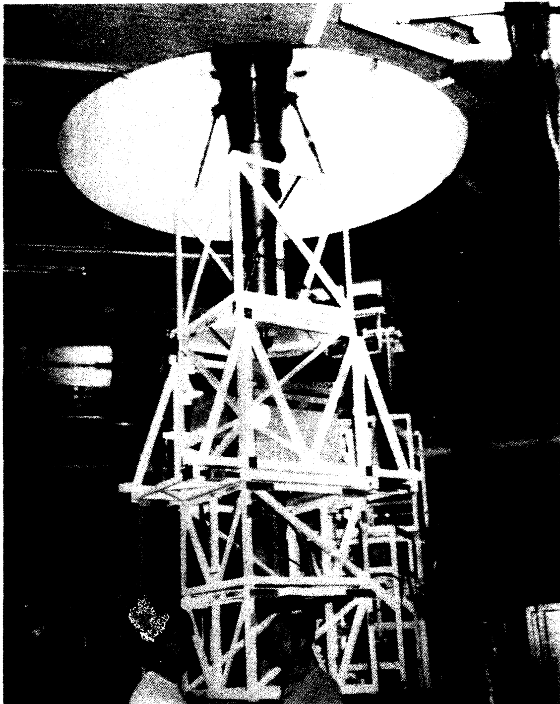
Figure 8. X-band 22-dBi horn test package and mounting table installed in the pedestal room focal point f_3 .
