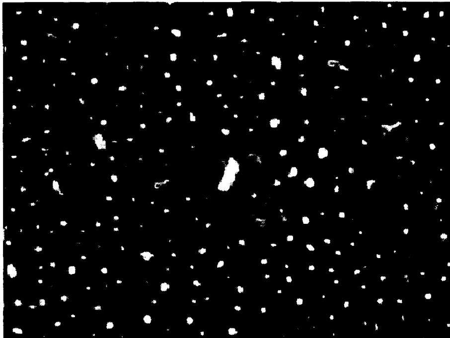
Figure 3f : Secondary electron image of the dirty surface of Cu(100) corresponding to Auger spectra in 3(c) and 3(d). Full scale (horizontal) is 1.2 \mu m.
