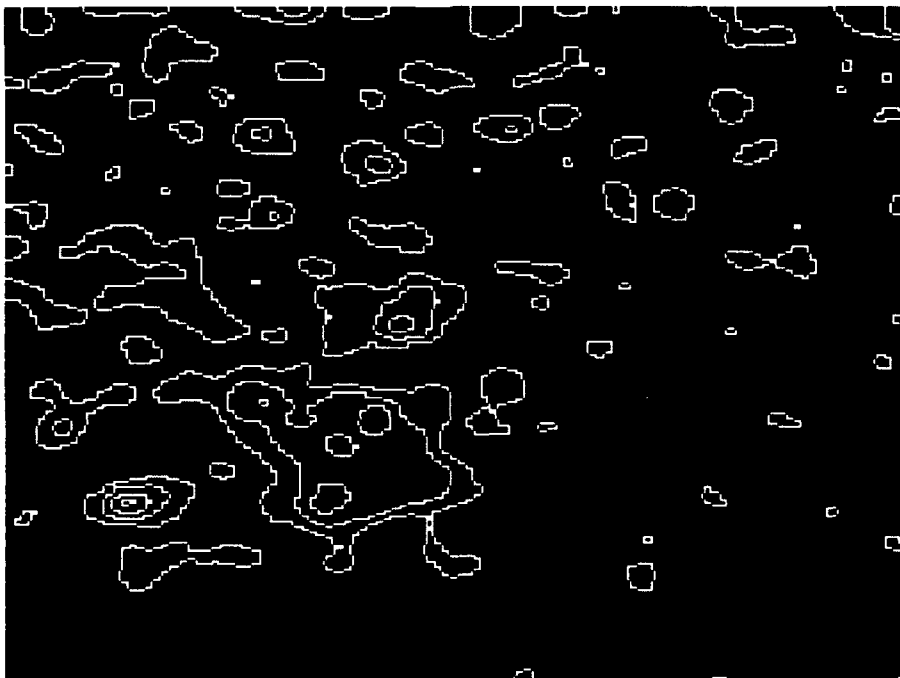
Figure 6f : Fe Auger electron micrograph contour map of 0.33 ML Fe/Cu(100) supersurface islands. The image is 150 nm full scale (horizontal) and is from the image in 6e.
