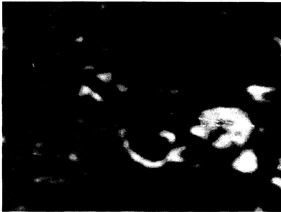
Figure 7c: Fe Auger electron micrograph of 1.7 ML Fe/Cu(100) subsurface islands. The image is 150 nm full scale (horizontal) and is from the identical area as Figs. 7a and 7b.
