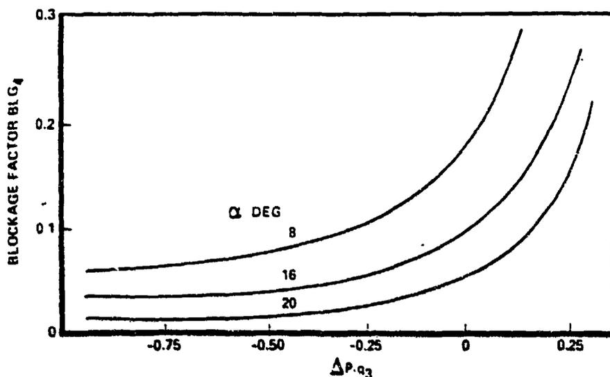
Figure 59 - Curve Fits of Blockage Factor for Diffuser Angles (Ref. 3)
