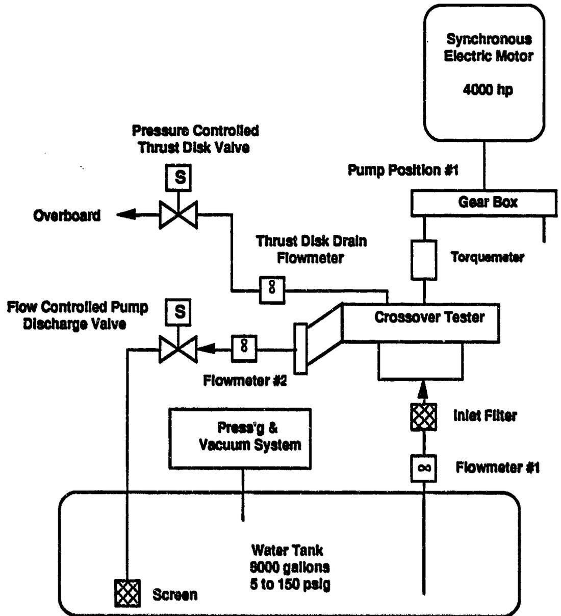
8000 gallon tank through the tester and returned to the tank in a recirculation mode. The tank pressurizing and vacuum systems were capable of maintaining a constant pressure at the pump inlet during the head versus flow maps and could also ramp the inlet pressure to less than 5 psia during the suction performance runs.
