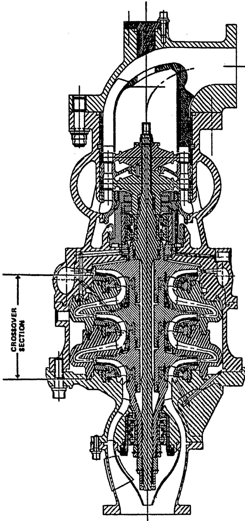
Figure 1 - MK49 Fuel Turbopump Cross-Section
