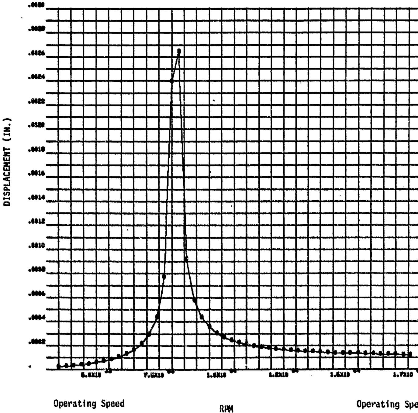
Figure 21 - Impeller Tip Deflections in Air
