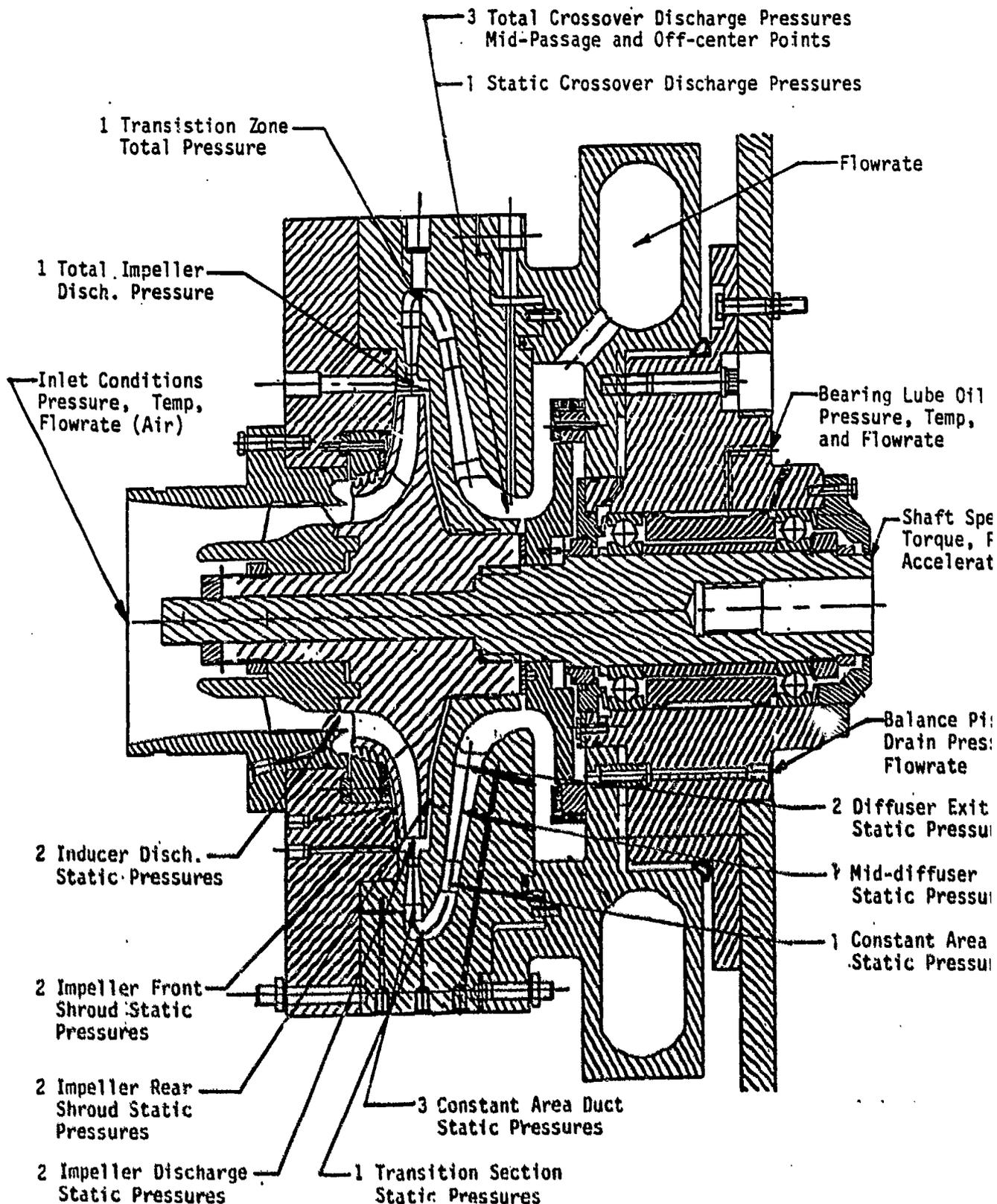
Table 7 - Air Test Instrumentation List
