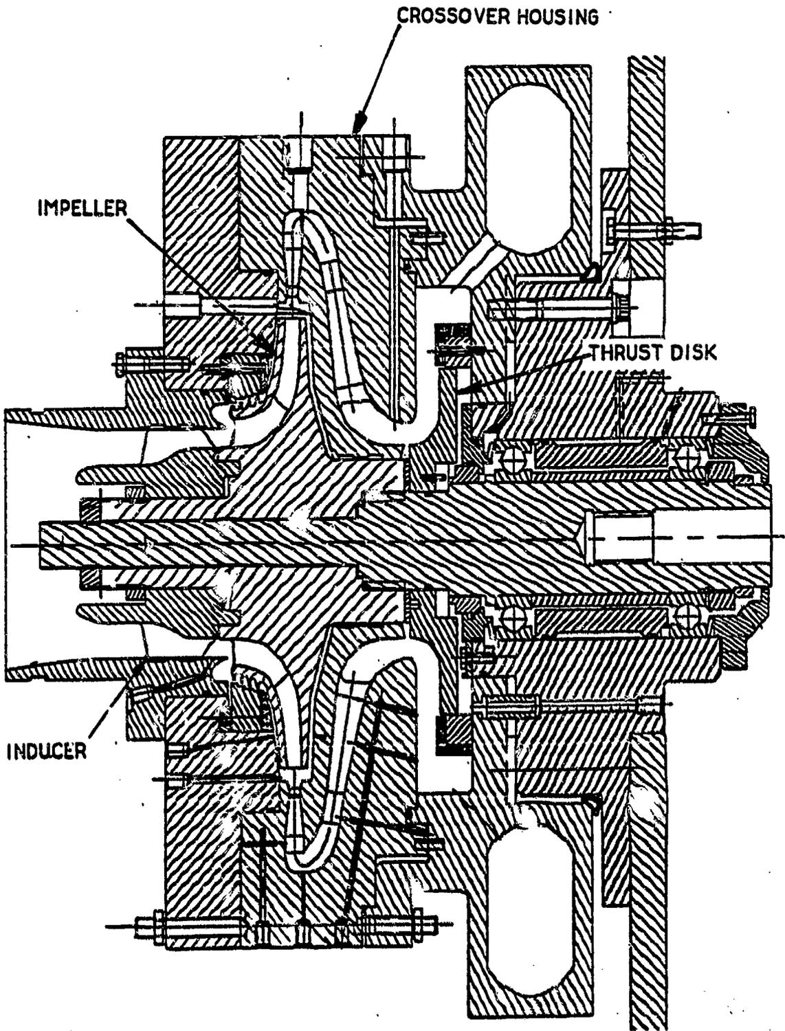
Figure 3 - Existing SSME HPFTP Tester Hardware
