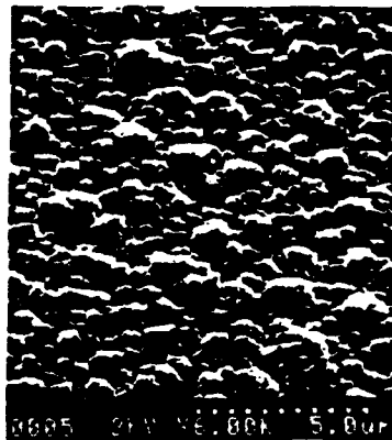
Fig. 2. SEM of 0.33%CH 4 /99.67%H 2 homoepitaxial (100) diamond after 6 hours.
