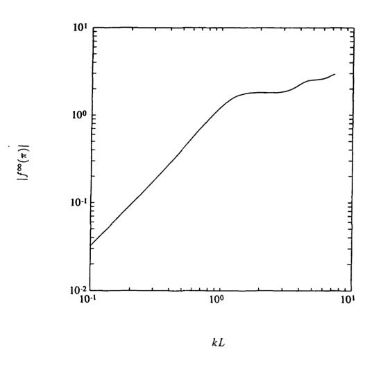
Figure 4.4: Backscattered form function of a Rigid Ten to One Ellipse:  $\theta_0 = \frac{\pi}{2}$  (direction of incidence along the minor axis). Both exact solution and approximate solution from the FMM are plotted.
