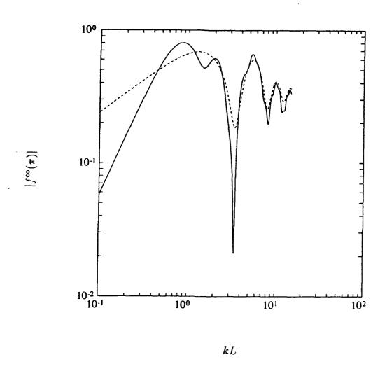
Figure 4.13: Backscattered form function of a Rigid Clover:  $\theta_0 = \pi/6$ . The dashed curve is from the physical optics approximation, and the solid curve is from the FMM under soft boundary conditions.
