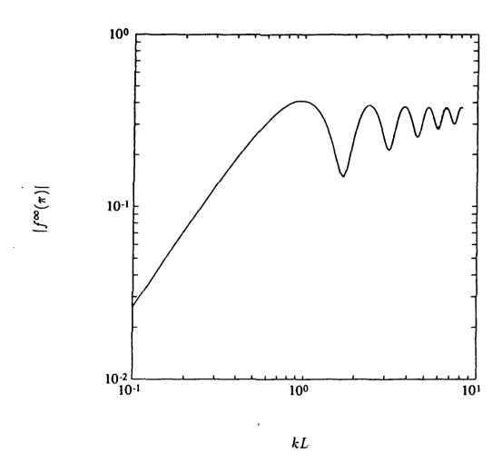
Figure 4.5: Backscattered form function of a Rigid Two to One Ellipse:  $\theta_0 = 0$  (direction of incidence along the major axis). Both exact solution and approximate solution from the FMM are plotted.
