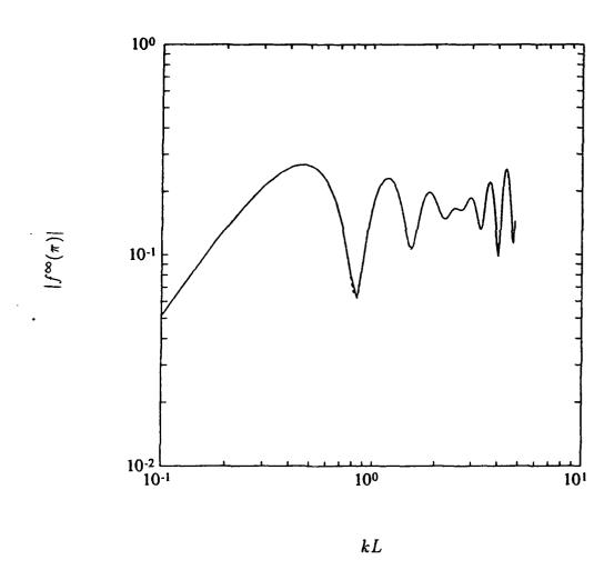
Figure 4.6: Backscattered form function of a Penetrable Two to One Ellipse:  $\theta_0 = 0$  (direction of incidence along the major axis). Both exact solution and approximate solution from the FMM are plotted. The material parameters are  $\frac{\rho_1}{\rho} = 2$  and  $\frac{c_1}{c} = 1.05$
