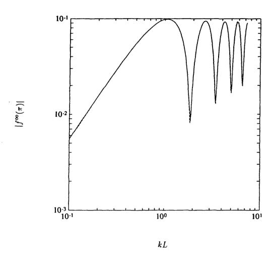
Figure 4.3: Backscattered form function of a Rigid Ten to One Ellipse:  $\theta_0 = 0$  (direction of incidence along the major axis). Both exact solution and approximate solution from the FMM are plotted.
