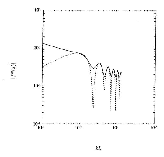
Figure 4.9: Backscattered form function of a Soft Square:  $\theta_0 = \frac{\pi}{4}$  (direction of incidence from the corner of the square). The dashed curve is from the physical optics approximation, and the solid curve is from the FMM under soft boundary conditions
