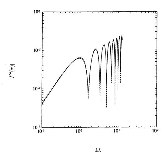
Figure 4.11: Backscattered form function of a Weakly Scattering Square:  $\theta_0 = 0$  (direction of incidence from the side of the square). The dashed curve is from the DWBA, and the solid is from the FMM. The material parameters are  $\frac{\rho_1}{\rho} = 1.05$  and  $\frac{c_1}{c} = 1.05$ .
