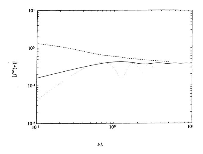
Figure 4.14: Backscattered form function from a 2:1 Ellipse.  $\theta_0 = 0$ . The solid curve is is from the physical optics approximation, the dashed curve is from the exact solution under soft boundary conditions, and the dotted curve is from the exact solution under rigid boundary conditions. This illustrates the fact that the physical optics solution will not necessarily accurately predict the level of the nulls.
