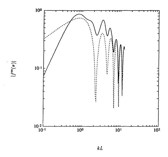
Figure 4.8: Backscattered form function of a Rigid Square:  $\theta_0 = \frac{\pi}{4}$  (direction of incidence from the corner of the square). The dashed curve is from the physical optics approximation, and the solid curve is from the FMM under rigid boundary conditions.
