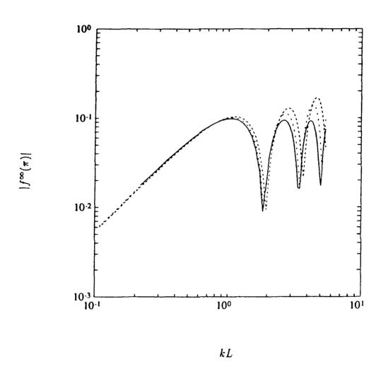
Figure 4.1: Backscattered form function of a Rigid Ten to One Ellipse:  $\theta_0 = 0$ . The solid curve is from the FMM using 16 modes, the dashed curve uses cylindrical weighting functions using 16 modes, and the dash-dotted curve uses cylindrical weighting functions using 22 modes.
