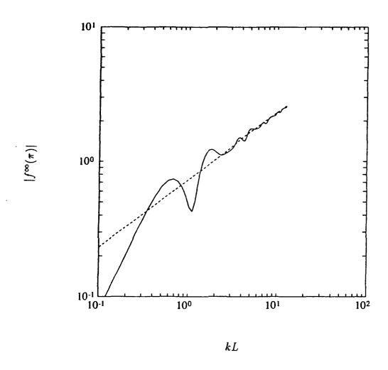
Figure 4.10: Backscattered form function of a Rigid Square:  $\theta_0 = 0$  (direction of incidence from the side of the square). The dashed curve is is from the physical optics approximation, and the solid curve is from the FMM under soft boundary conditions.
