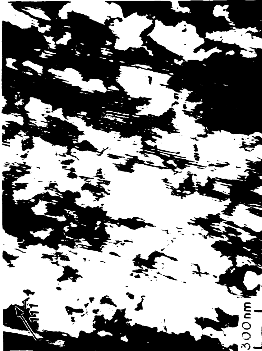
FIGURE 33. High density of extended faults and SISF debris.
