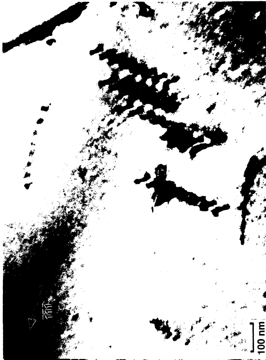
FIGURE 31. Typical SISF coupled pairs.
