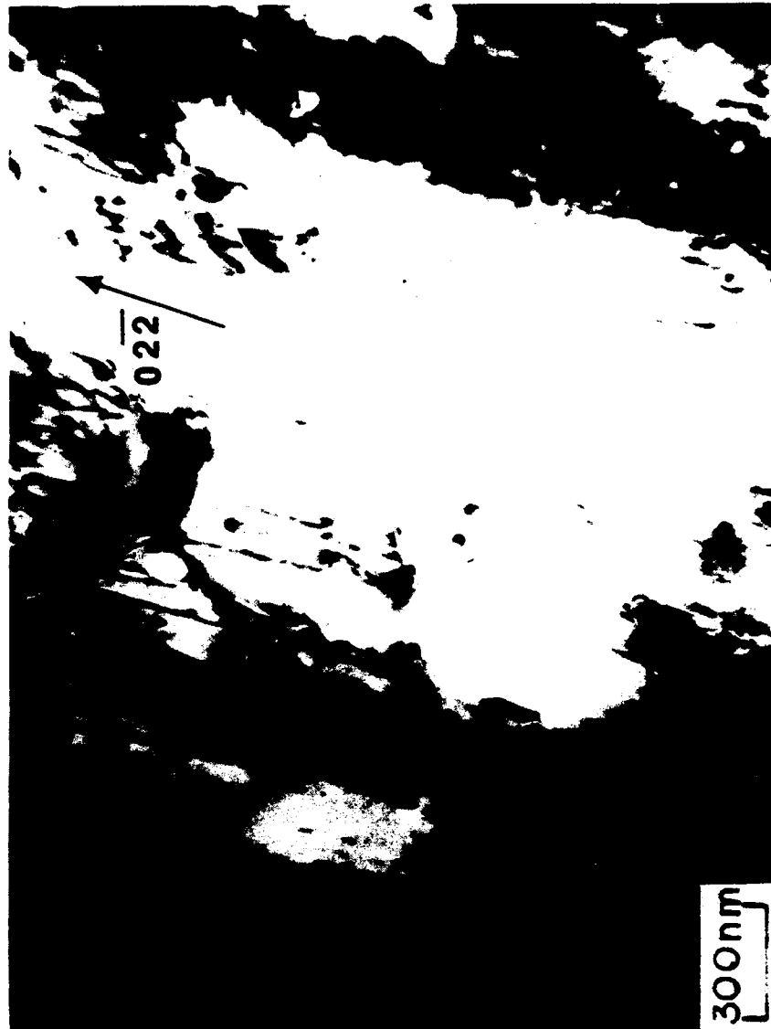
FIGURE 62. Faults and some dislocations invisible.
