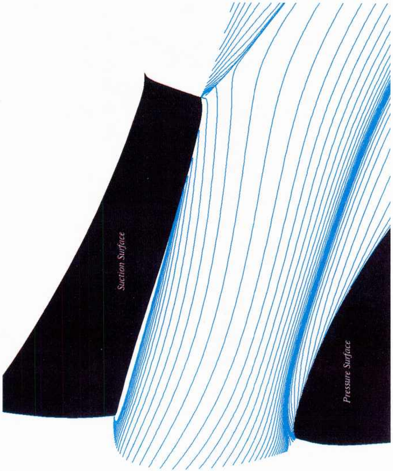
4.17 Predicted Particle Paths, One Grid Point from the Rotor Blade Hub
