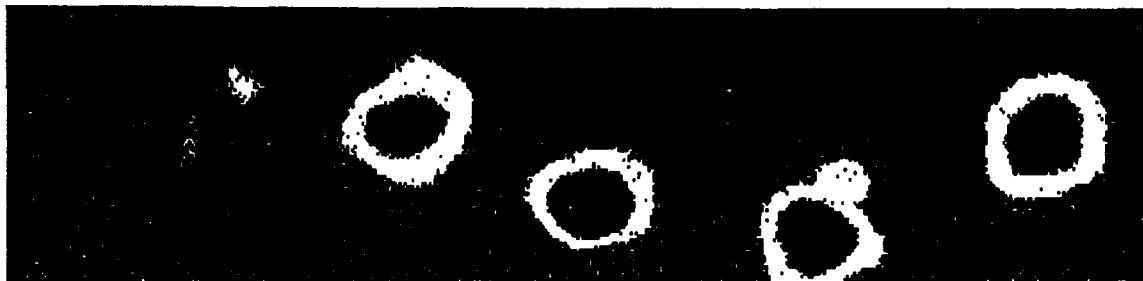
Figure 60. C-scan obtained by SAM of one column of defects found in as-fired curved ceramic specimen (G2) containing 0.105-inch-square by 0.005-inch-thick planar defects. The area shown represents a 0.5-inch by 2.25-inch area on the specimen.
