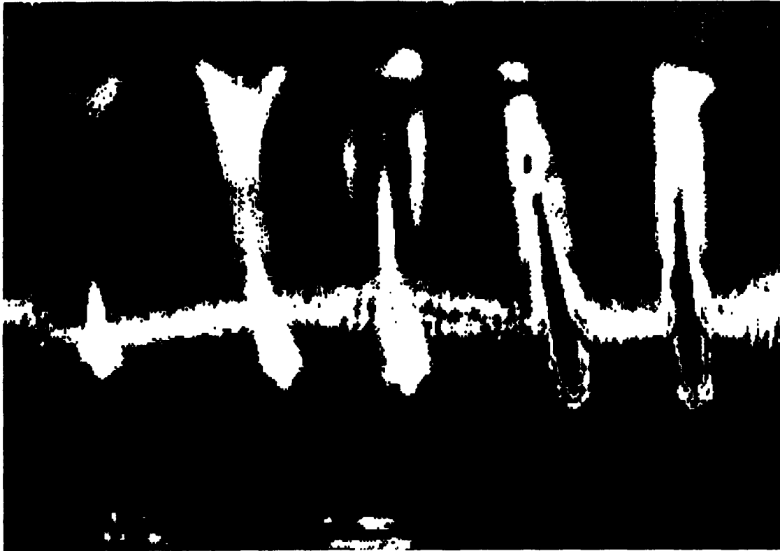
Figure 57. C-scan obtained by SAM of one column of defects found in as-fired curved ceramic specimen (D2) containing 1-inch-long by 0.028-inch-diameter rod-shaped defects. The area shown represents a 2.25-inch by 1.5-inch area on the specimen.
