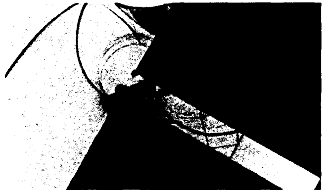
Fig. 2 Shadow-schlieren photography: oblique penetration of a shock wave in a tunnel entrance. Vortices at the entrance reduce the afterflow behind the passing shock front.
