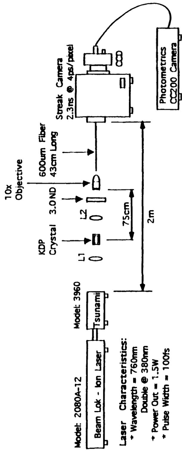
Figure 8 Schematic of Fiber Dispersion Test Layout
