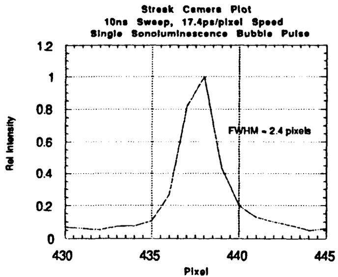
Figure A-7 Single Sonoluminescence Event Streak Camera Image
