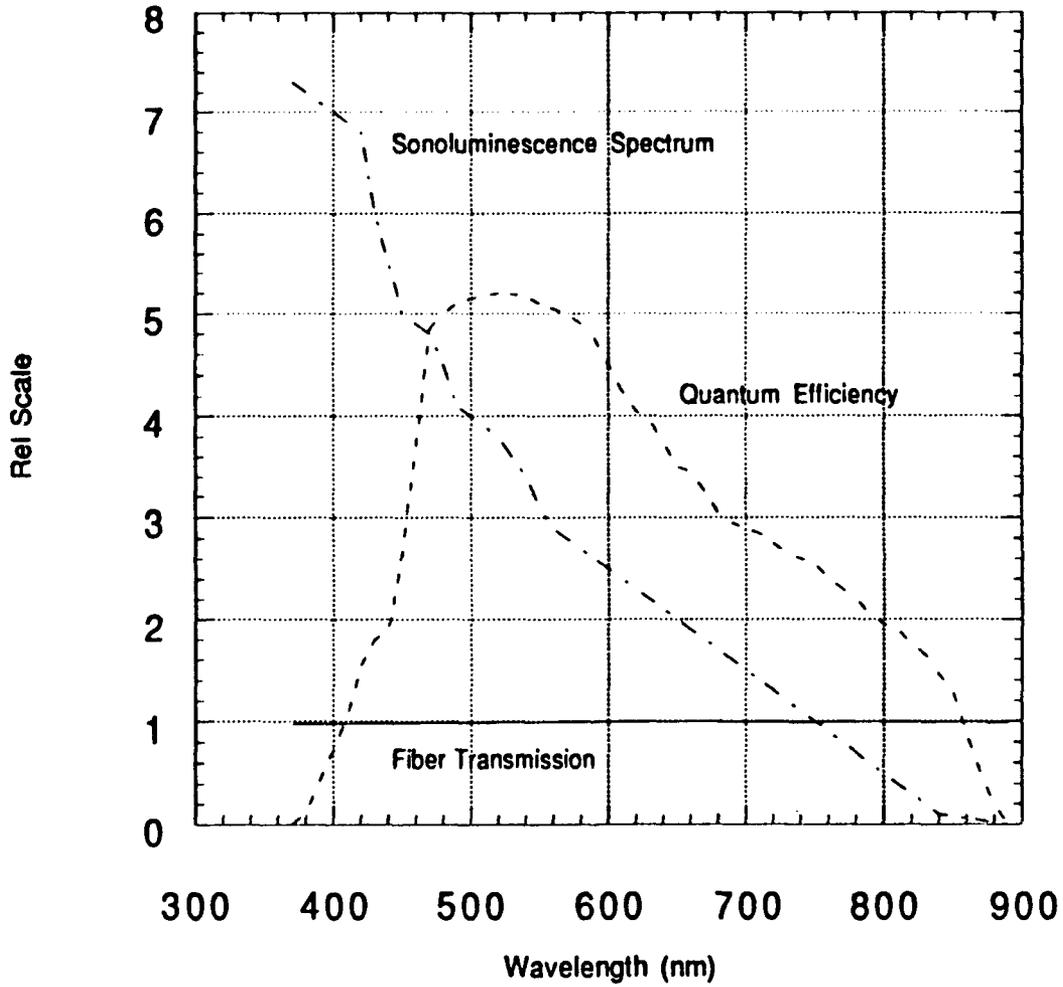
Figure 15 Relative Plot of Sonoluminescence Spectrum, Streak Camera
