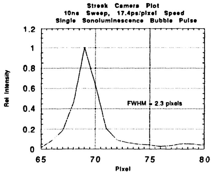
Figure A-3 Single Sonoluminescence Event Streak Camera Image
