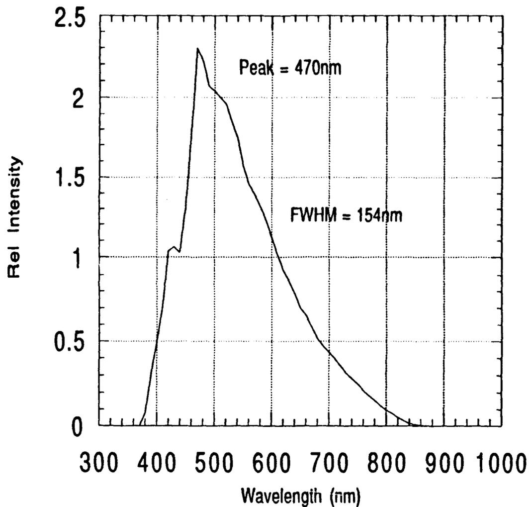
**Figure 16 Streak Camera System Effective Response Curve For
