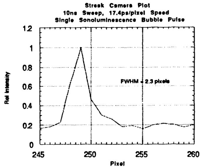
Figure A-4 Single Sonoluminescence Event Streak Camera Image
