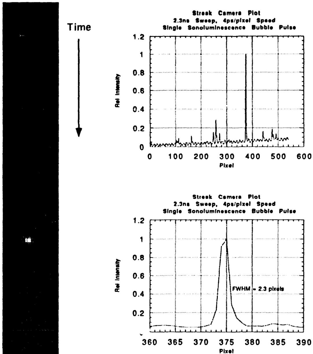
Figure B-1 Single Sonoluminescence Event Streak Camera Image and Intensity Plots, File #95s1
