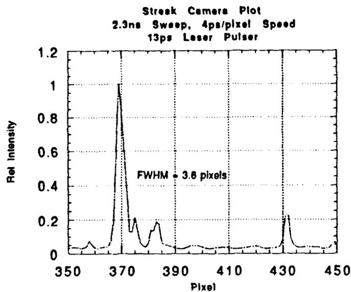
Figure 7 13 ps Laser Pulser Streak Camera Image and Intensity Plots, File #p8
