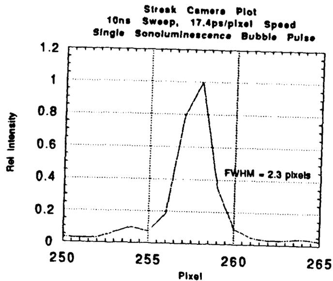
Figure 5 Single Sonoluminescence Event Streak Camera Image and Intensity Plots, File #10s2
