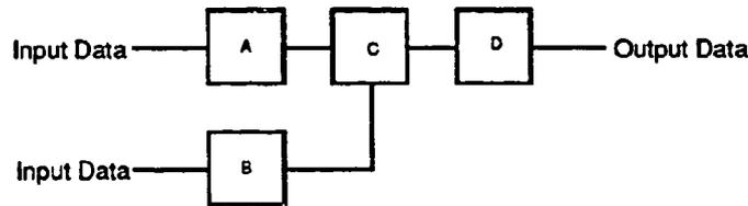
Figure 15. Pipelined Topology
