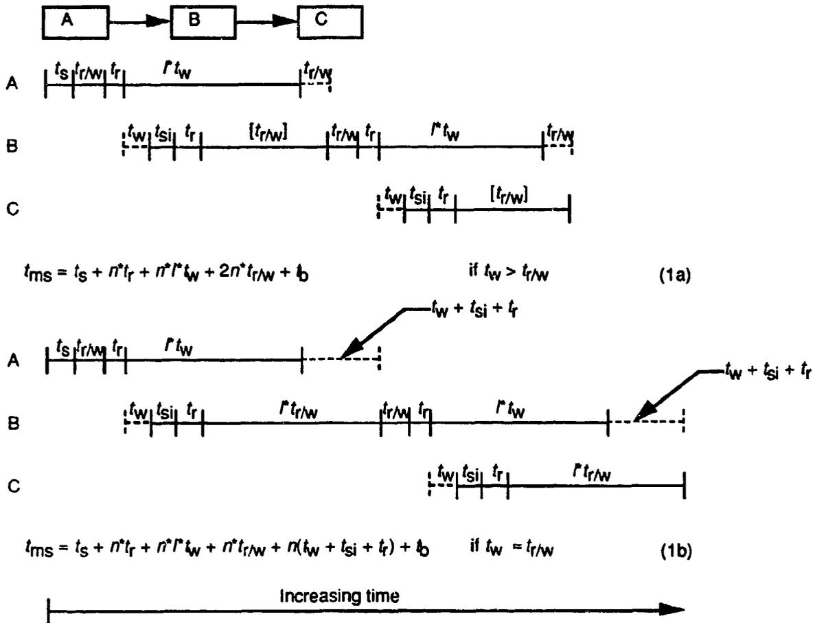
Figure 3. Timing Diagrams Used to Derive Equations 1
