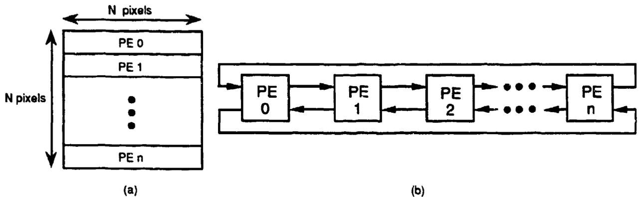
Figure 22. Mapping AS4 onto a Ring Network
