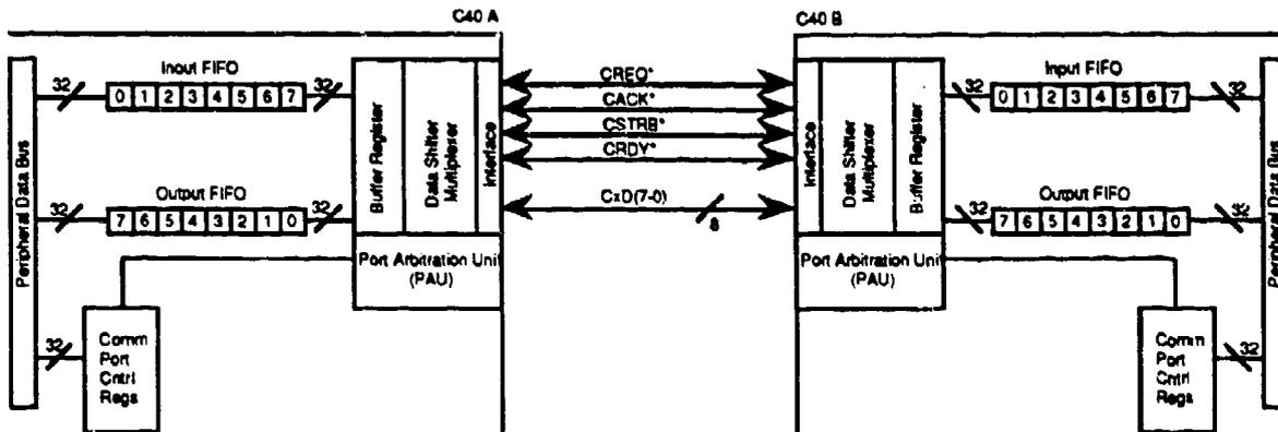
Figure 2. Details of Communication Port Hardware [2]
