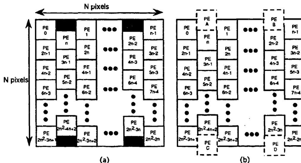
Figure 18. Image Partitioning and Extra Processor Overlap
