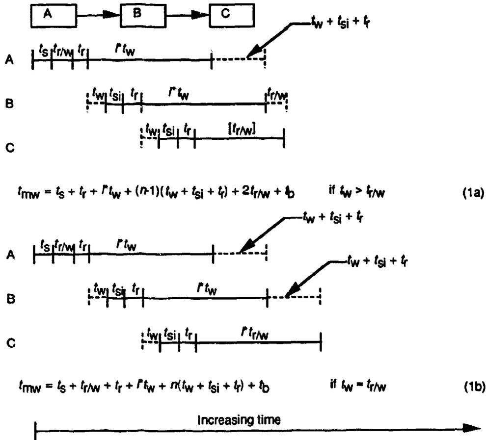
Figure 7. Timing Diagrams Used to Derive Equations 2
