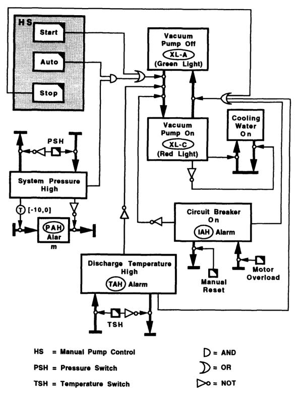
Figure 2. Specification of Standby Vacuum Pump
