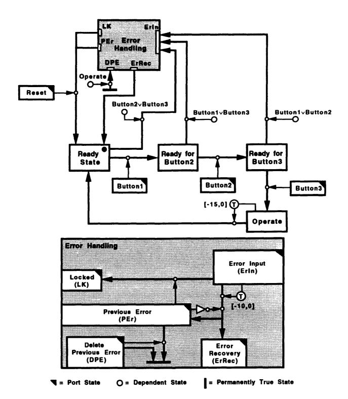
Figure 1. HMS Machine Specification of Sequential Lock
