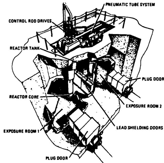
Figure 1. Cutaway view of AFRRI TRIGA reactor.
