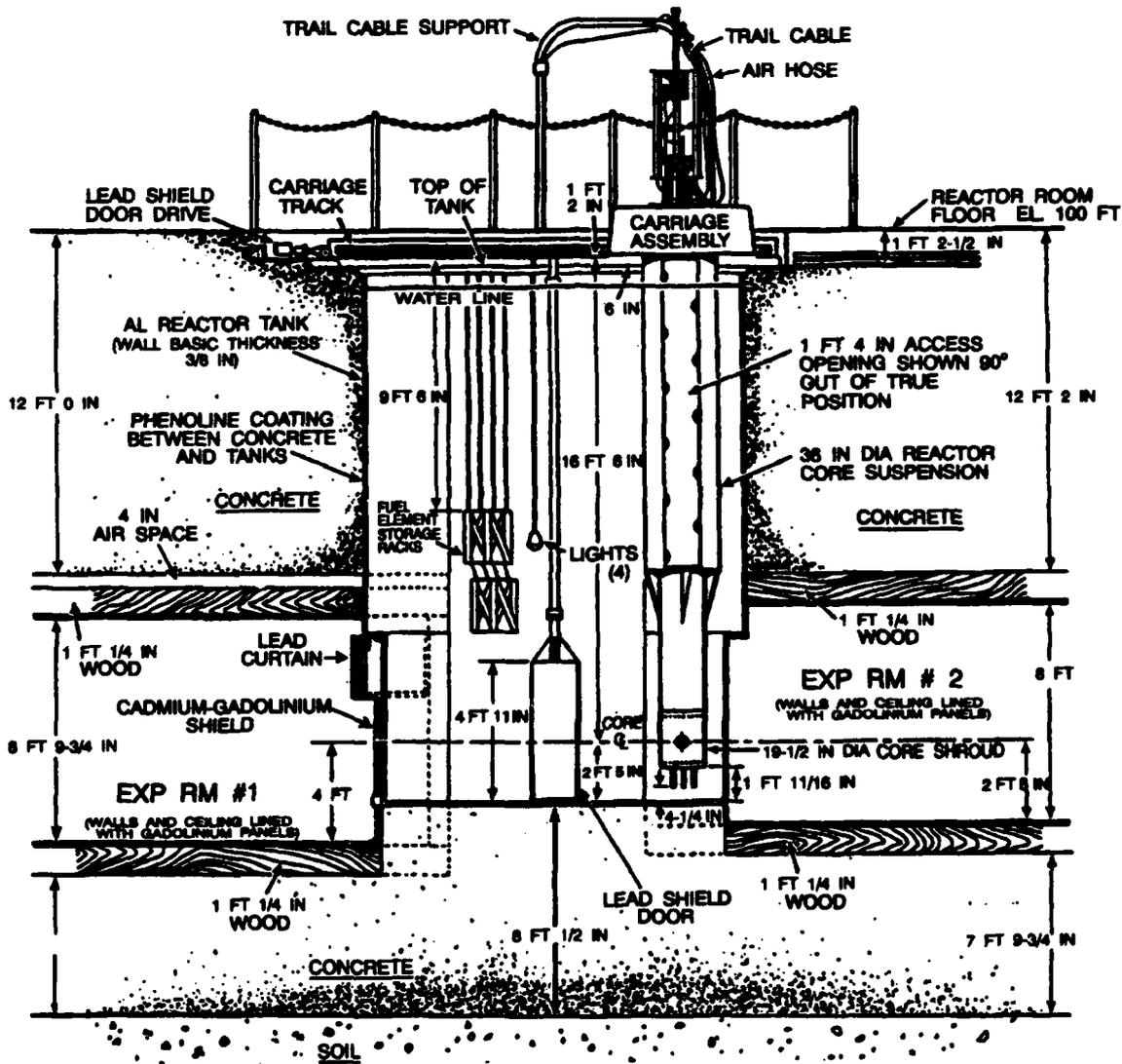
Figure 5. Side view of reactor and exposure facilities.
