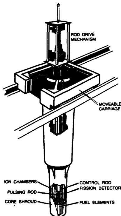
Figure 4. Reactor core.
