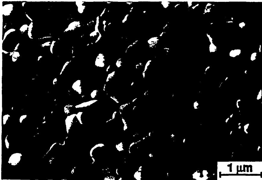
FIG. 11. SEM micrograph of polished and etched mullite/ zirconia/alumina sample sintered at 1500°C for 2 h.
