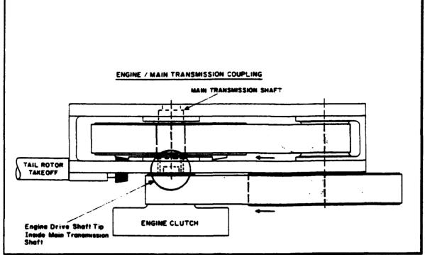
Figure 11. Schematic of Engine and Transmission Coupling
