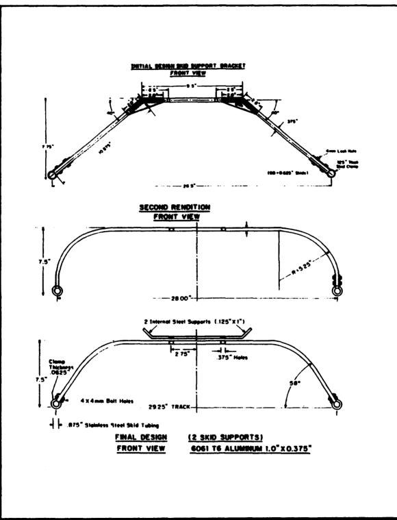
Figure 13. Three Renditions of Skid Support Design
