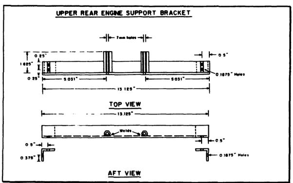
Figure 23. Upper Engine Mount Schematic
