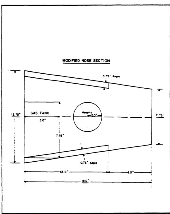
Figure 25. Schematic of Enlarged Nose Compartment
