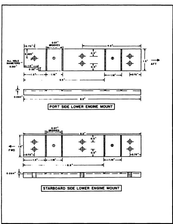
Figure 17. Schematic of Lower Engine Mounts
