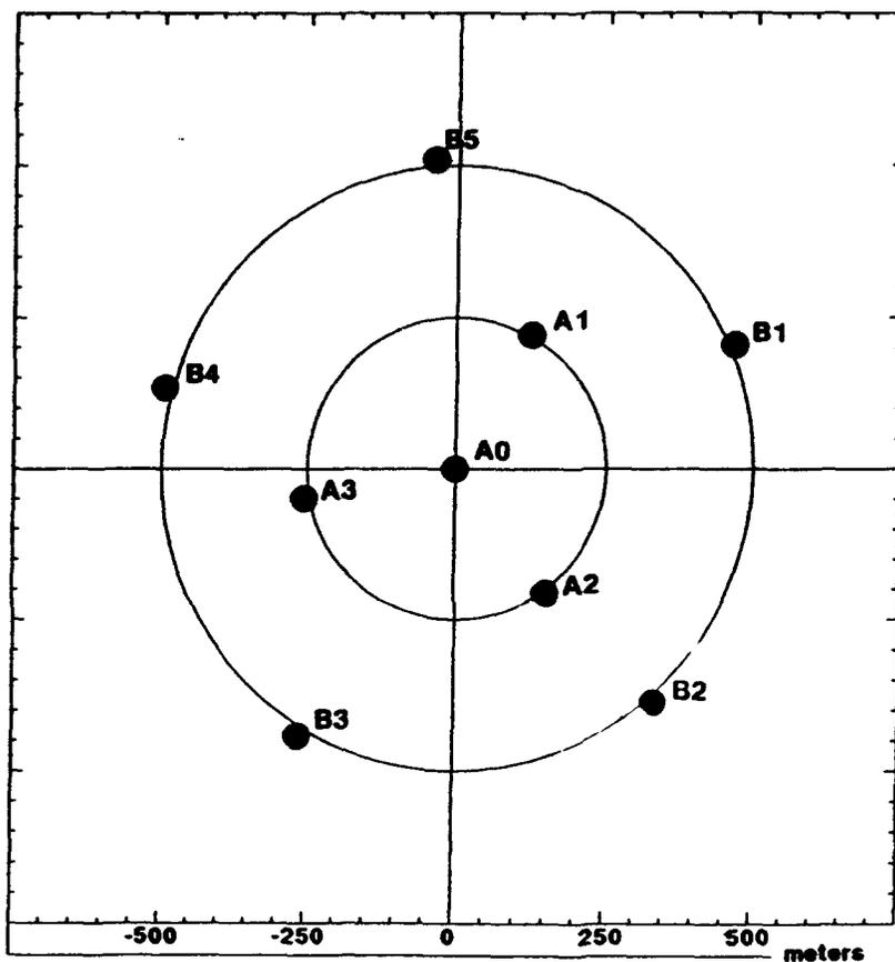
Fig. 7.5.2. Configuration of the new Spitsbergen small-aperture array.
