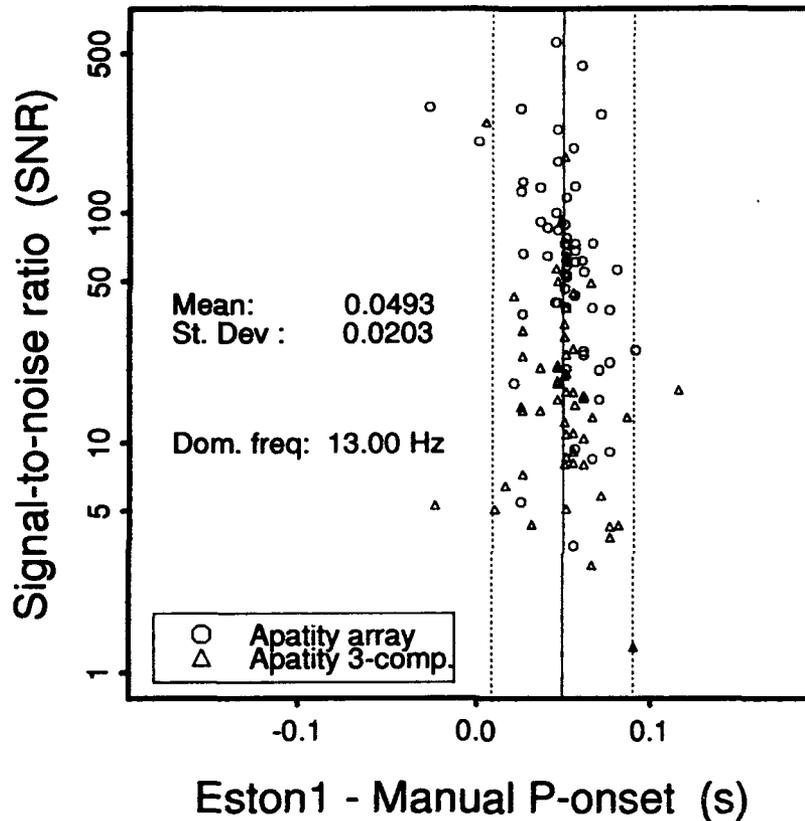
**Fig. 7.2.7.** This figure show the time differences between the automatic P-onsets from ESTON1 and the manual pick at both Apatity stations (APA0 and APZ9) as a function of signal-to-noise ratio (SNR). Compared to Fig. 7.2.5 the x-axis is strongly expanded. Notice that P-phases at APZ9 (triangles) generally have lower SNR. The average dominant frequency of these P-phases is 13 Hz.
