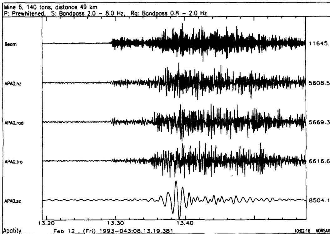
**Fig. 7.2.3.** Seismograms from an event at mine VI recorded at the Apatity array. The source-receiver distance is 49 km. The only difference from the traces of Fig. 7.2.2 is that the upper trace is the array beam steered with steering delays corresponding to the slowness and azimuth of the P-arrival. Notice that in this case the S-phase is much more emergent than the S-phase of Fig. 7.2.2.
