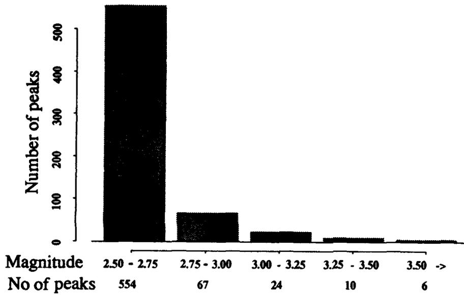
Fig. 7.4.4. Histogram showing the distribution of peaks on the network threshold trace for the four-month monitoring experiment.
