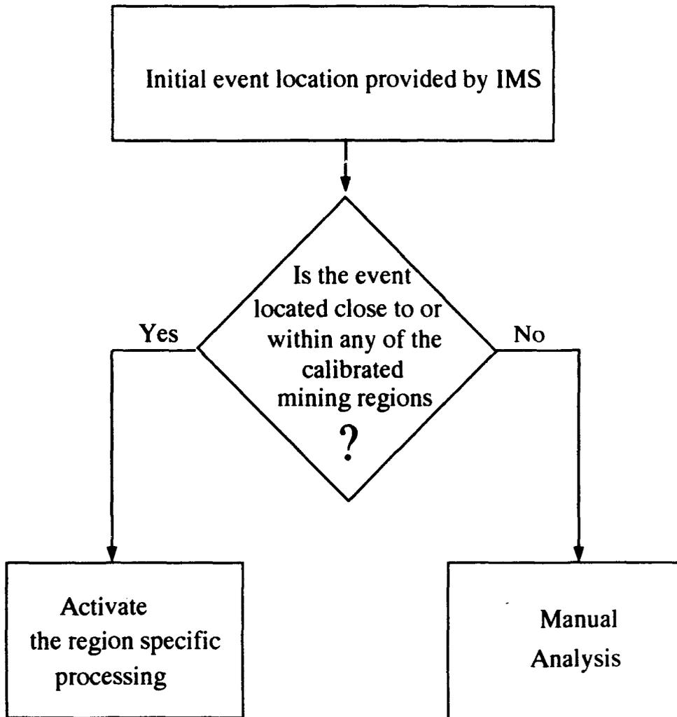
**Fig. 7.3.1.** Schematic view of the principle behind intelligent post-processing of seismic events.
