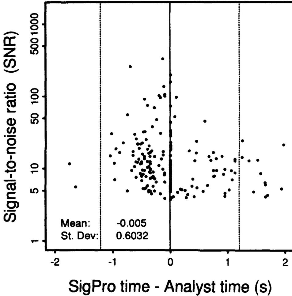
Fig. 7.6.3. The figure shows differences between arrival times as determined by SigPro and arrival times determined by the analyst during review, plotted versus SNR, for Pn phases used by IMS to form events during the evaluation period 26 April - 2 May 1993. The mean value of the arrival time differences is marked by a solid vertical line, whereas the two strippled lines denote  $\pm 2$  standard deviations.
