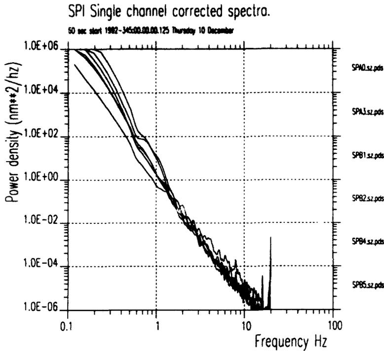
**Fig. 7.5.3a.** Noise spectra corrected for system response for the Spitsbergen array for 6 vertical channels. The spectra are based on one minute of data at 00.00 hours GMT on day 345, 1992. The power density is in nm<sup>2</sup>/Hz.
