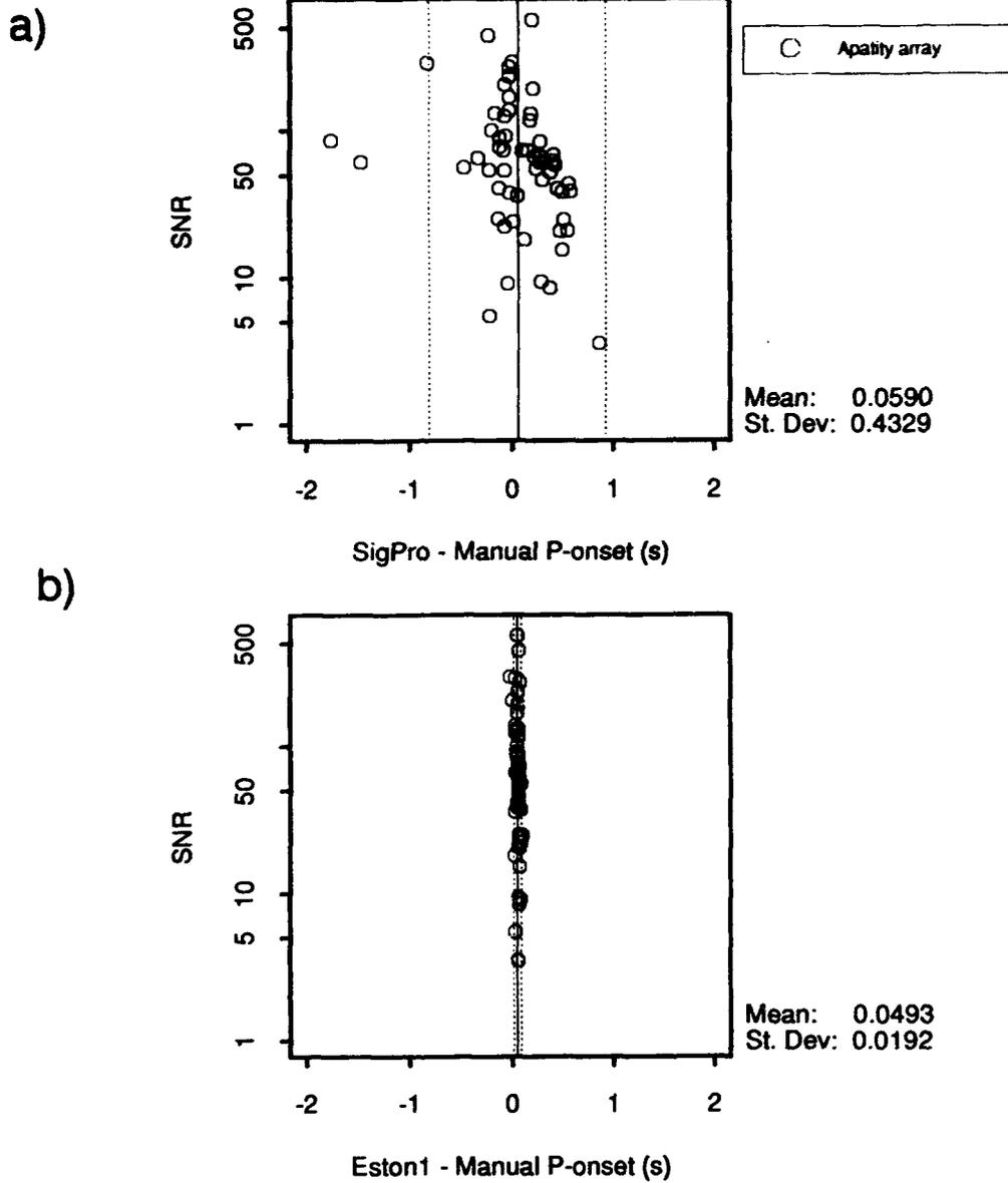
**Fig. 7.2.5.** These two plots show the time differences between the automatic P-onsets and the manual pick at APA0 as a function of signal-to-noise ratio (SNR) on the prewhitened beam. All 58 P-observations are included. Figure **a)** shows the time differences between the automatic P-onsets from the IMS and the manual picks, whereas figure **b)** shows the time differences between the automatic P-onsets from ESTON1 and the manual picks. The two vertical dotted lines represent  $\pm\sigma$ .
