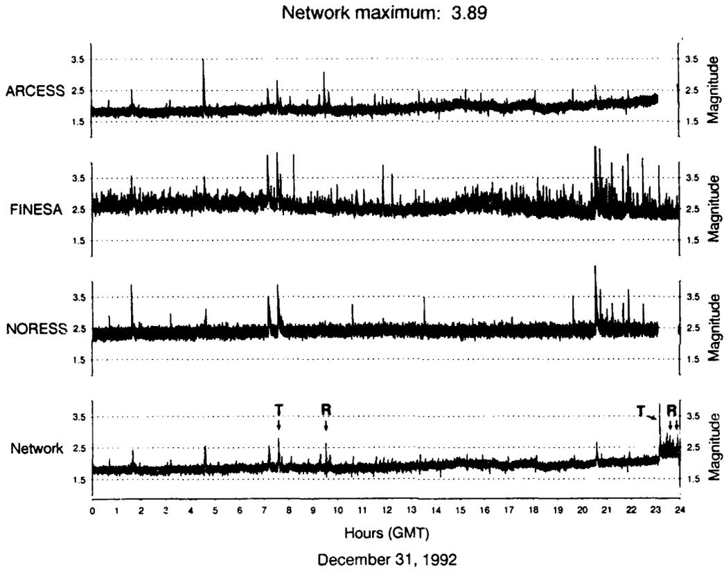
**Fig. 7.4.5.** Threshold plot for 31 Dec 92 (see Fig. 7.4.3 for explanation). The small Novaya Zemlya event at 09.29 GMT is indicated.
