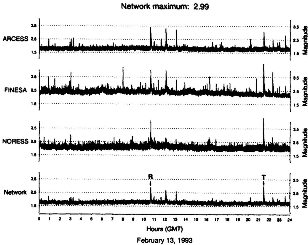
**Fig. 7.4.2.** Example of continuous threshold monitoring of Novaya Zemlya for one day (13 February 1993). A “threshold trace” is shown for each of the 3 arrays, and the combined network threshold trace is shown at the bottom. Note that the network threshold is well below magnitude 2.5 almost all the time.
