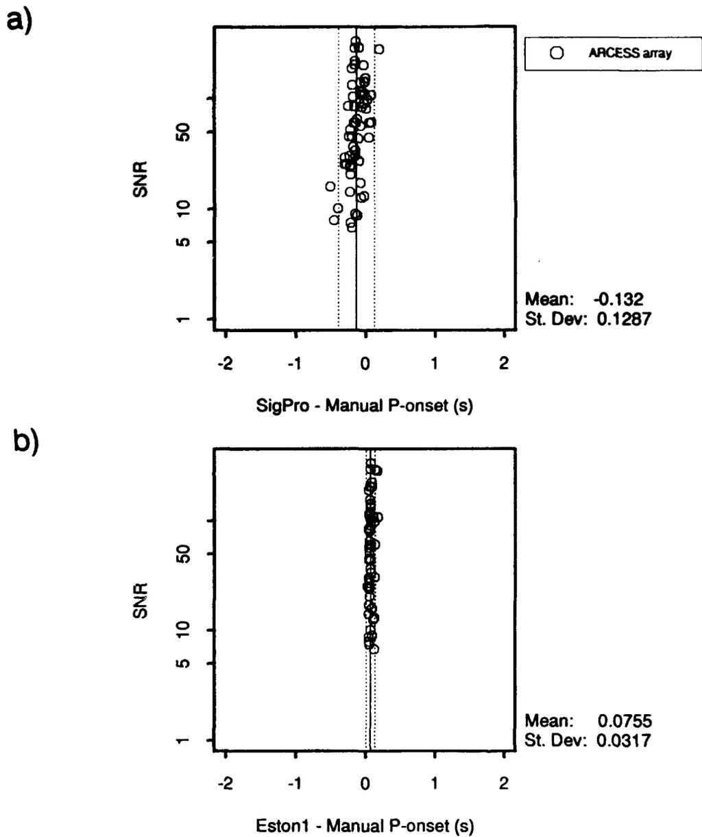
**Fig. 7.2.6.** Plots similar to those of Fig. 7.2.5, but in this case for Pn-onsets at ARCESS. For one of the Khibiny Massif events, the ARCESS array was not operational, and consequently only 57 P-phases were analyzed.
