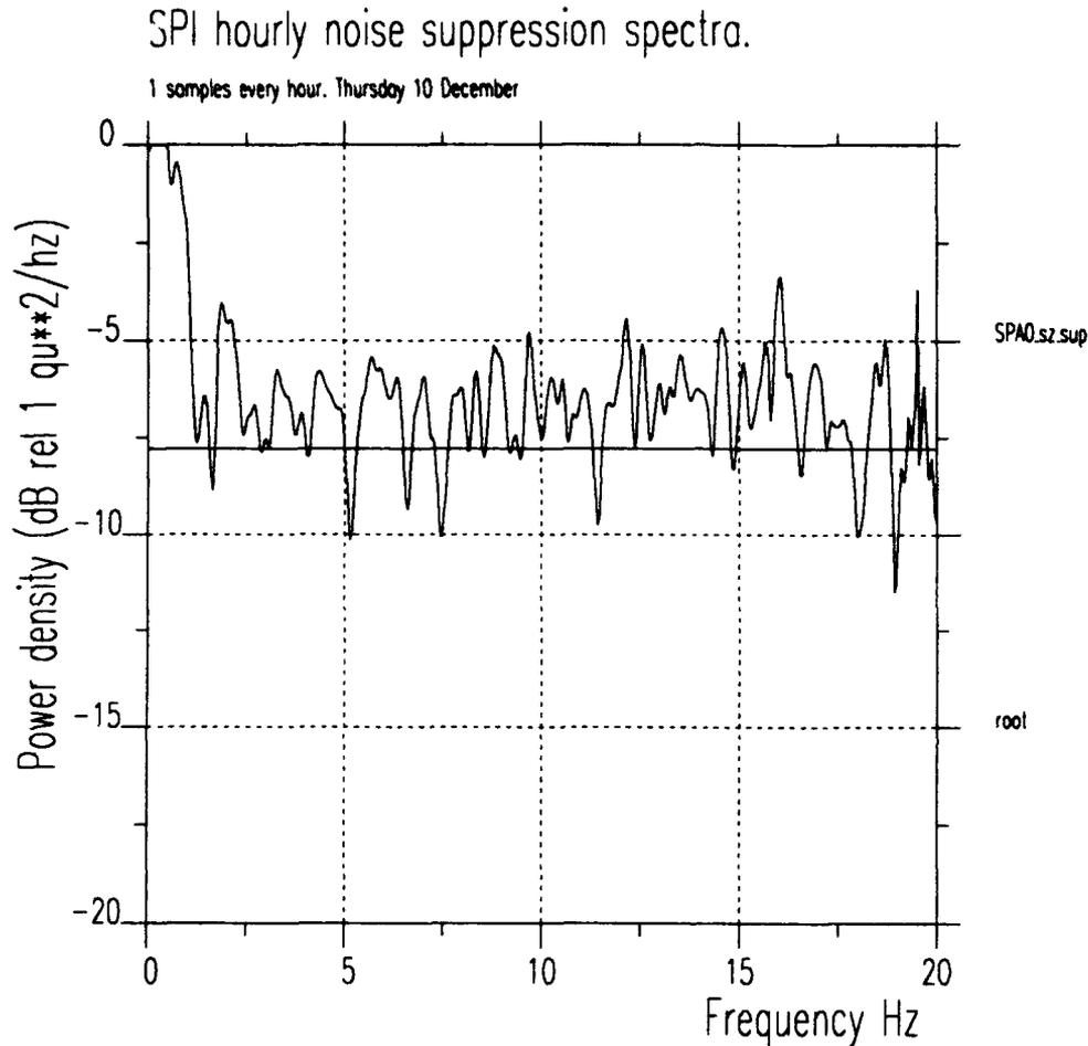
**Fig. 7.5.5.** Spitsbergen array noise suppression by beamforming for the initial geometry. The plot shows an average of 24 curves. To produce each of these curves, an infinite-velocity beam is formed and the spectrum for this beam is divided by the average of the single sensor spectra. The 24 curves result from one minute of data taken hourly between 00.00 and 23.00 hours GMT on day 345, 1992. The horizontal line at -8 dB represents  $\sqrt{N}$  suppression for 6 sensors.
