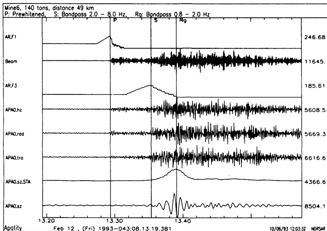
**Fig. 7.2.10.** The traces of this plot are similar to those of Fig. 7.2.9. The seismograms are Apatity array (APA0) recordings of the Mine VI event also shown in Fig. 7.2.3. The source-receiver distance is 49 km. Notice that the S-phase is much more emergent than the S-phase of Fig. 7.2.9, but the ESTON3 likelihood function still shows a clear peak at the S-onset.
