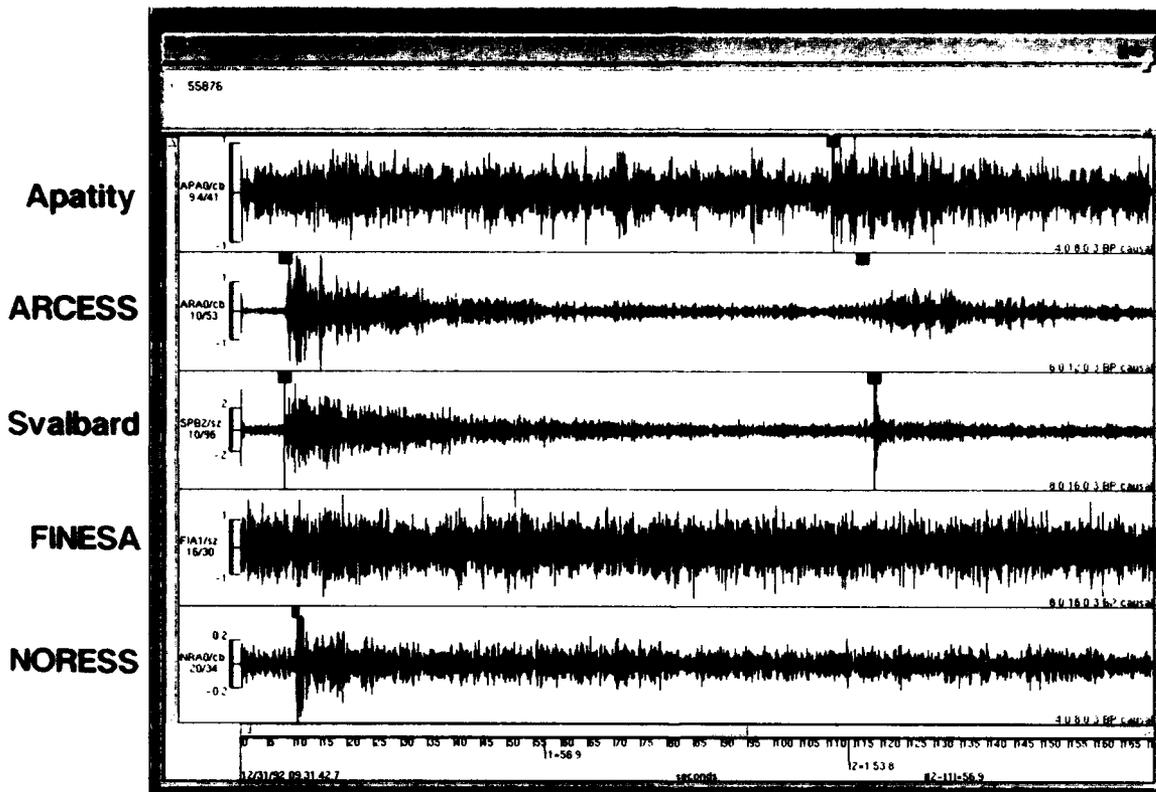
**Fig. 7.4.7.** Waveform plots for 5 regional arrays for the Novaya Zemlya event on 31 Dec 92. There are P-phase detections at ARCESS, Svalbard (Spitsbergen) and NORESS, and S-phase detections at Apatity, ARCESS and Svalbard.
