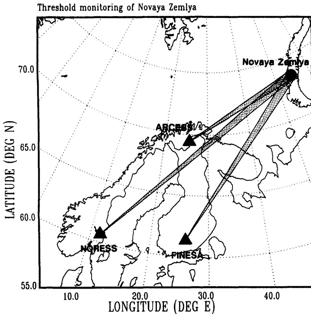
Fig. 7.4.1. Location of the target area (the northern Novaya Zemlya test site) for the monitoring experiment. The locations of the three arrays NORESS ( $\Delta = 2280$  km), ARCESS ( $\Delta = 1100$  km) and FINESA ( $\Delta = 1780$  km) are indicated.
