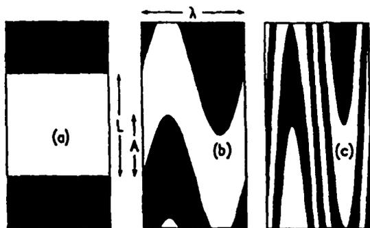
FIG. 1. Pattern of equally spaced sinusoidal steps used here. Black and white regions correspond to  $2 \times 1$  and  $1 \times 2$  domains, which are separated by single-layer steps. Step spacing  $L$ , wavelength  $\lambda$ , and amplitude  $A$  are indicated. (a)  $A=0$ , (b)  $A=0.6L$ , (c)  $A=3L$ .  $L$  and  $\lambda$  are the same in all three figures.
