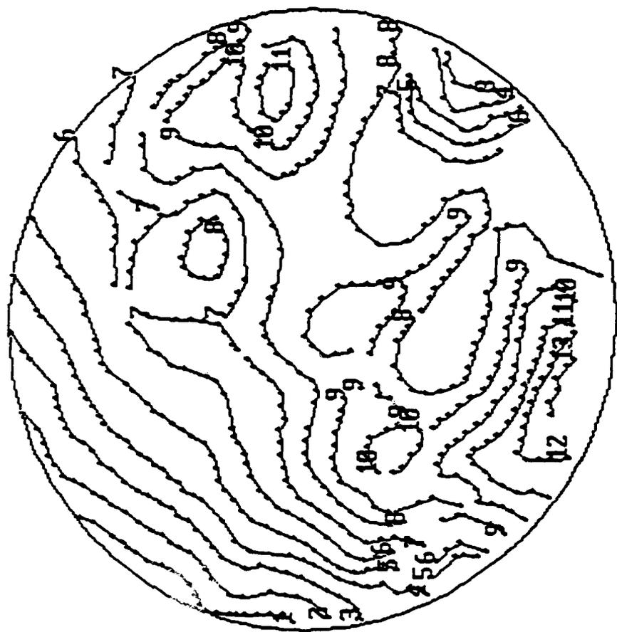
Figure 8. Fringe tracing or the digitized fringe data of the interferogram shown in figure 7.
