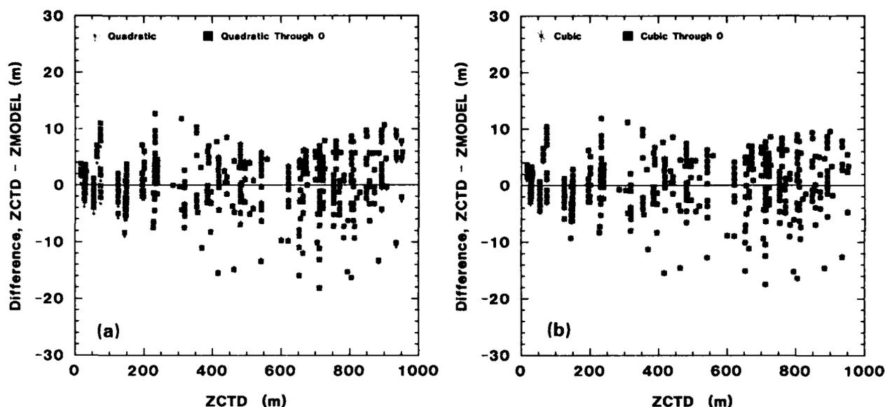
FIG. 4. The difference CTD depth minus AXBT depth plotted versus CTD depth for all CTD-AXBT pairs: (a) quadratic models from Table 6 for AXBT depth; (b) cubic models. A square indicates the model forced through 0; an asterisk indicates the model containing a constant. For all practical purposes, in both instances the depths calculated from the model forced through 0 and the model with a constant are the same.
