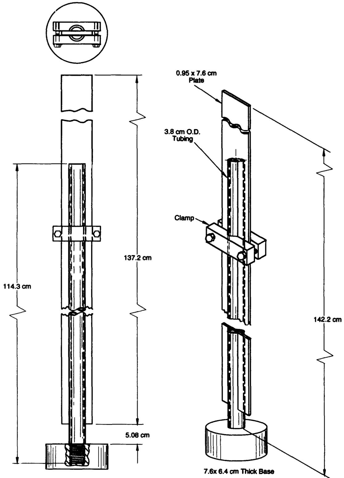
Figure 1. Temperature profile measuring device.
