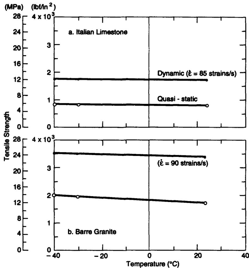
Figure 7. Effect of temperature and strain rate on the tensile strength.
