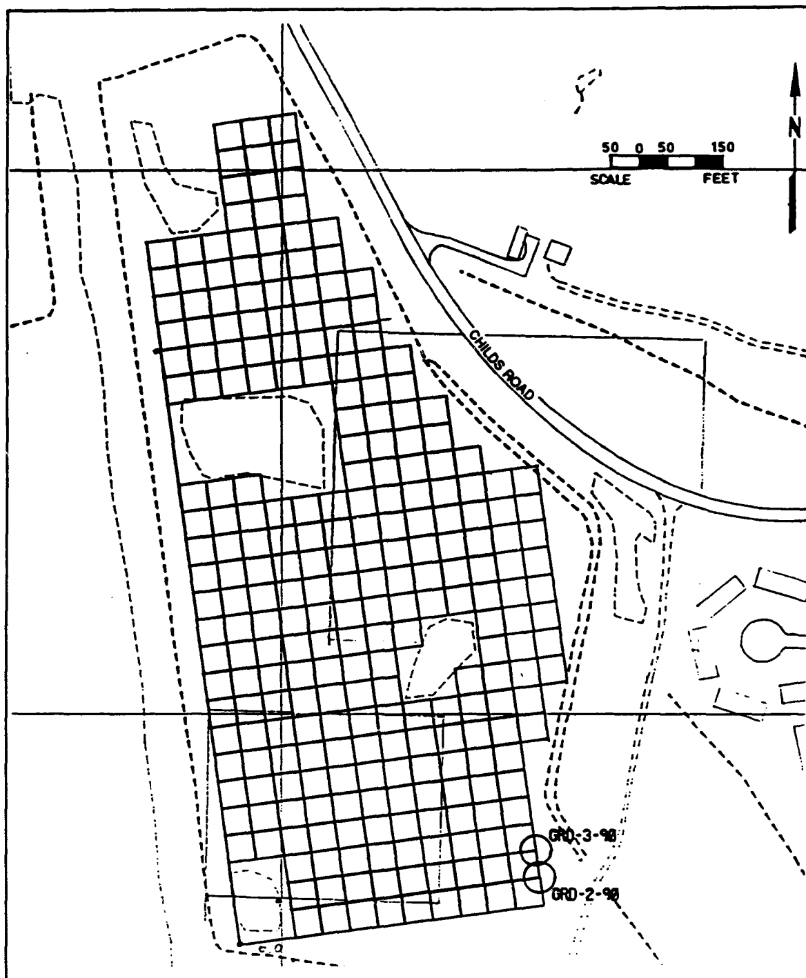
Figure 7. Outline of grid for geophysical survey of overall site
