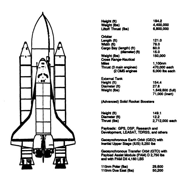
The typical mission length of the Space Shuttle is 7 days. Crew size varies between four and seven people per mission. The Space Shuttle system consists of the Orbiter, two reusable Solid Rocket Boosters (SRBs), and the External Tank. The launch site for the Shuttle is Cape Canaveral AFB and the landing site is located at Edwards AFB. Typical altitude of the Shuttle Orbiter is 135-320 nautical miles (NM).
