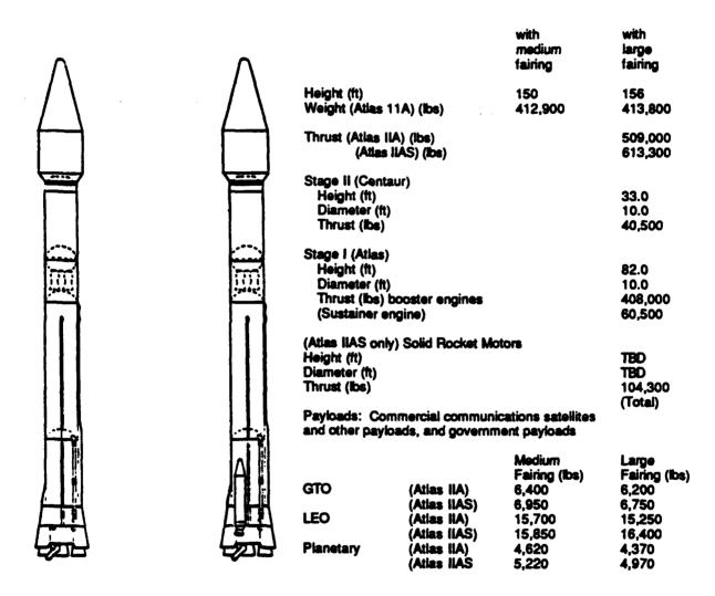
The Atlas IIA and IIAS are the same except that the Atlas IIAS has CTPB-fueled SRMs to provide greater lift capability. Both are derived from the Atlas II with an improved Centaur stage for providing greater thrust. The Centaur stage uses LH<sub>2</sub> and LO<sub>2</sub> and the Atlas stage uses LO<sub>2</sub> and RP-I for propellant.
