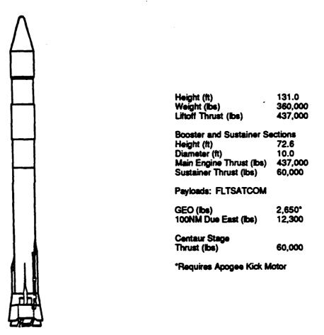
The Atlas Centaur was developed to provide launch services for geostationary payloads and heavy LEO payloads. The Atlas Centaur is equipped with more powerful main engines than other Atlas vehicles. The Centaur stage provides an additional 60,000 pounds of thrust.
