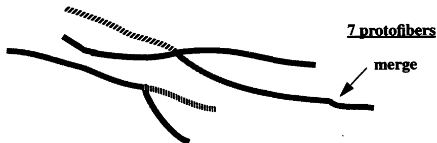
Figure 11: Protofibers from Figure 10 after short branches have been removed.
