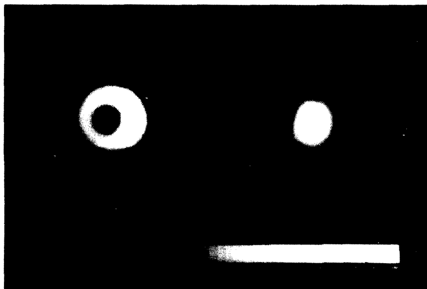
← Figure 2: Comparison of the directional characteristics of two eddy current testing probes: Left: The standard commercial probe exhibits a loss of sensitivity at the centre. Right: The probe developed at BAM has maximum sensitivity at the centre.
