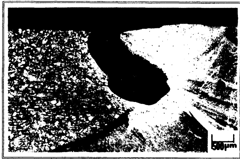
SMAW weld cross-section showing fusion line pitting attack
