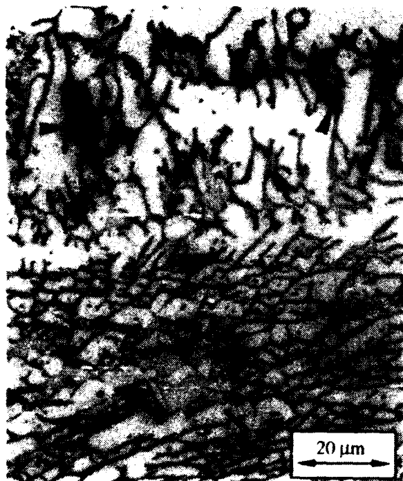
Figure 7 Optical micrograph showing the preferential precipitation of \sigma -phase (dark) in "austenitic" regions in a super duplex weld metal.
