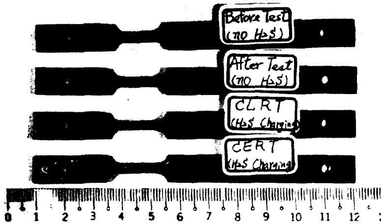
Figure 6. Micrograph of failed specimens under CERT and CLRT
