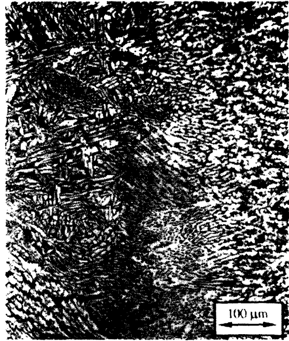
Figure 2 Super duplex weld metal with a microstructure consisting of regions with a "normal duplex" microstructure (left) and "austenitic" regions in which the ferrite (dark phase) had a lacy or vermicular appearance.
