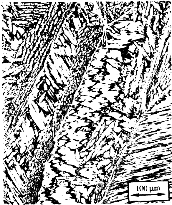
Figure 1 Typical microstructure of duplex weld metal with Widmanstätten type austenite in ferrite (dark phase).
