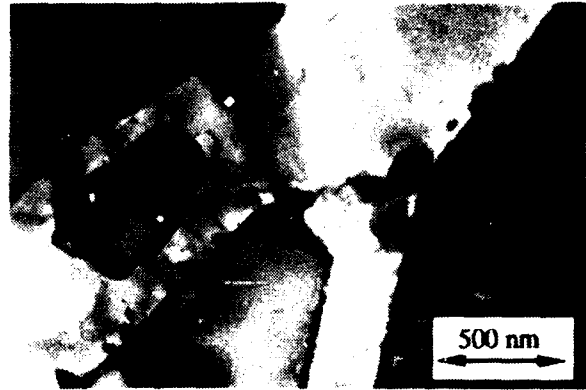
Figure 6 TEM images of R-phase particles at ferrite/austenite boundaries formed in a duplex weld metal during isothermal heat treatment.
