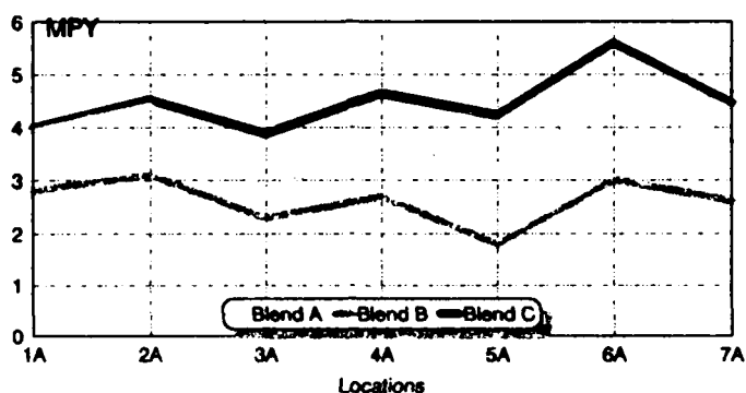
Pitting Rates of Three Types of Inhibitor Bases
