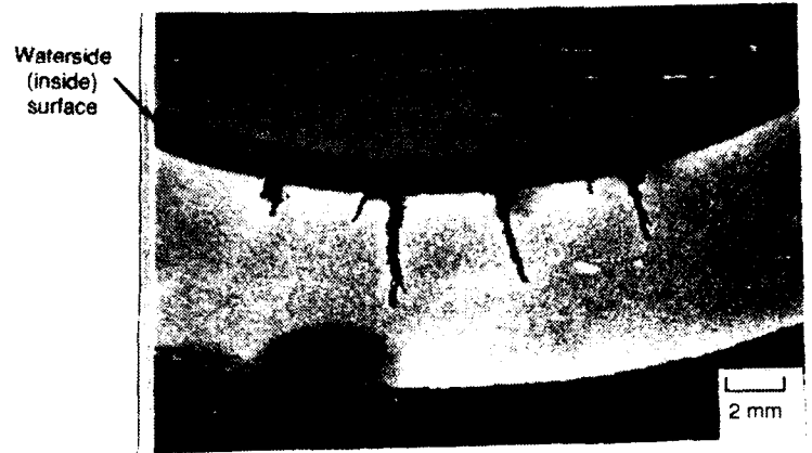
(b) Cross-sectional view of the boiler tube in (a)
