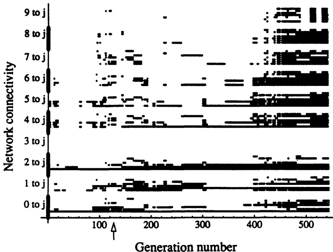
Figure 7. Different network topologies explored by GNARL during the first 540 generations on the enable-trigger problem. The presence of a link between node  $i$  and  $j$  at generation  $g$  is indicated by a dot at position  $(g, 10 * i + j)$  in the graph. Note that because node 3 is the output node, there are no connections from it throughout the run. The arrow designates the point of transition between the first two training sets.
