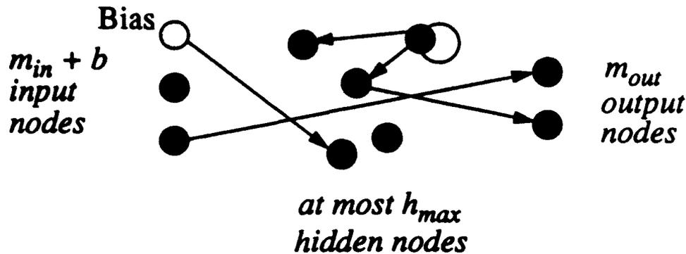
Figure 4. Sample initial network. The number of input nodes ( $m_{in}$ ) and number of output nodes ( $m_{out}$ ) is fixed for a given task. The presence of a bias node ( $b = 0$  or  $1$ ) as well as the maximum number of hidden units ( $h_{max}$ ) is set by the user. The initial connectivity is chosen randomly (see text). The disconnected hidden node does not affect this particular network's computation, but is available as a resource for structural mutations.
