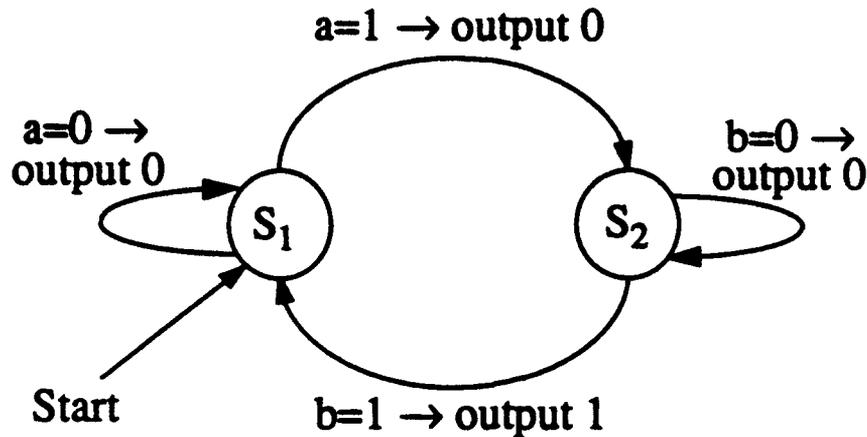
Figure 5. An FSA that defines the enable-trigger task [39]. The system is given a data stream of bit pairs  $\{(a_1, b_1), (a_2, b_2), \dots\}$ , and produces an output of 0's and 1's. To capture this system's input/output behavior, a connectionist network must learn to store state indefinitely.
