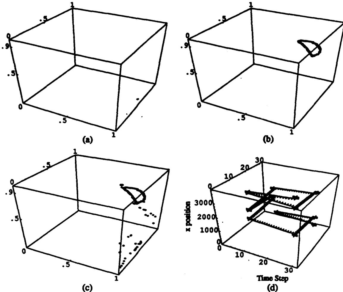
*Figure 2: Limit behavior of a network for the ant problem. Graphs show the state of the output units Move, Right, Left. (a) Fixed point attractor that results for sequence of 500 "food" signals; (b) Limit cycle attractor that results when a sequence of 500 "no food" signals is given to network; (c) All states visited while traversing the trail; (d) The x position of the ant over time when run on an empty grid.*
