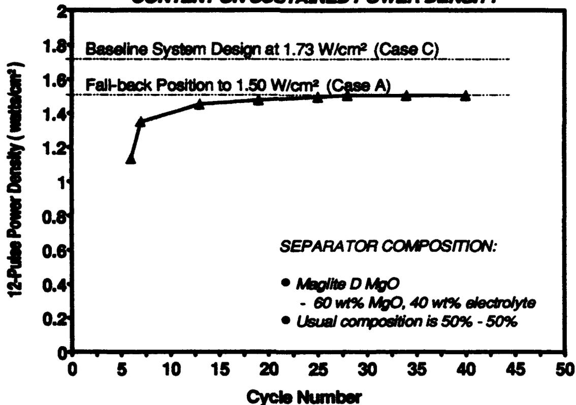
Figure 21. The electrolyte content of the separator can be reduced to 40%. Further reduction will result in unacceptably low power densities.
