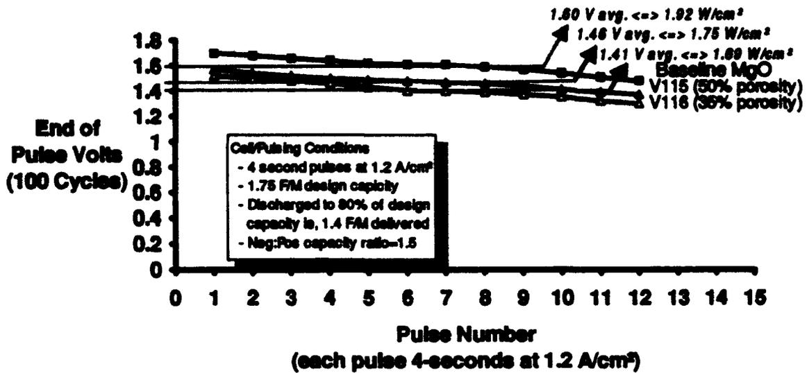
Figure 4. Both dimensionally stable AlN separators tested have exceeded the 100 cycle goal at average power densities which satisfy projected system requirements.
