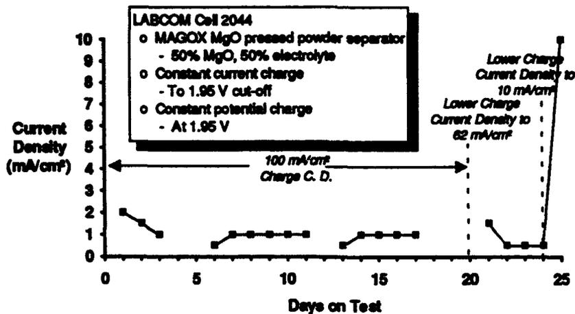
Figure 13. Stable Final Currents Have Been Maintained Over Extended Cycling. Rapid Cell Failure Occurred While Testing a Charge Current Density Below 50 mA/cm<sup>2</sup>.
