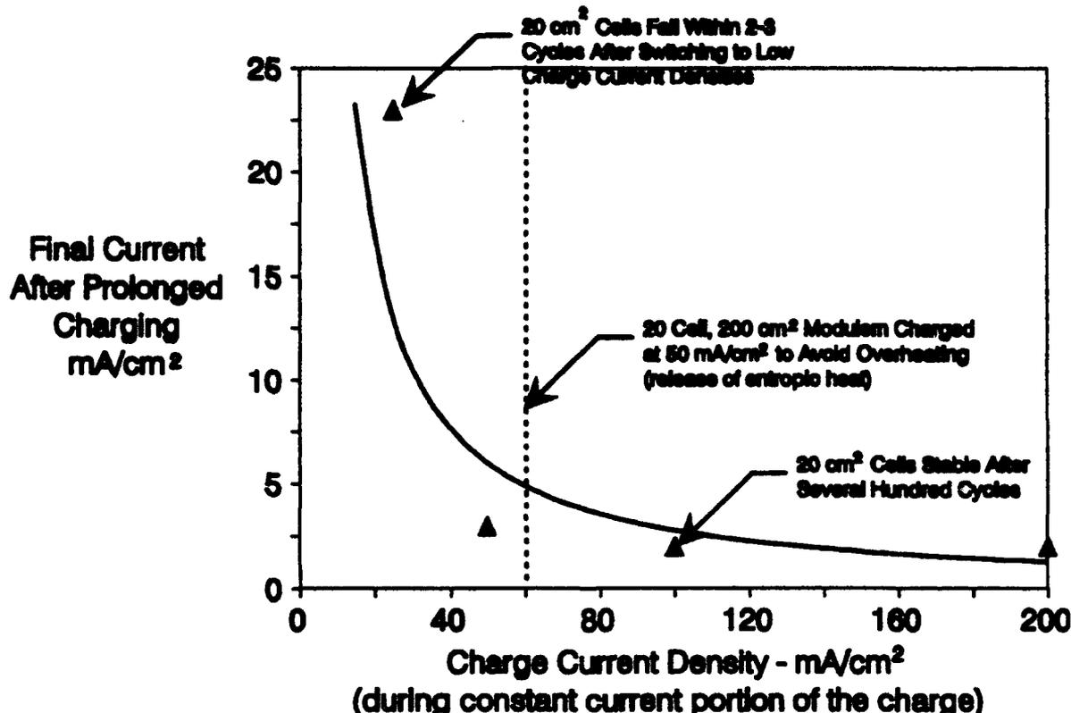
Figure 20. Charge Current Densities Below 50 mA/cm<sup>2</sup> Can Result in Rapid Cell Failure. Full Area Modules Must Have Sufficient Radial Heat Transfer Capability to Support this Charge Rate.
