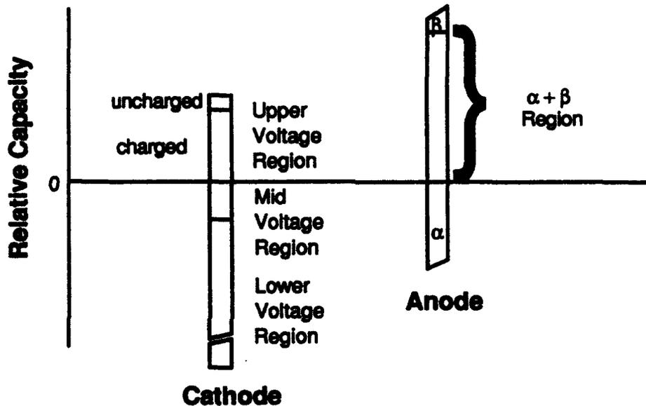
Figure 14. Cell Electrochemical Design
