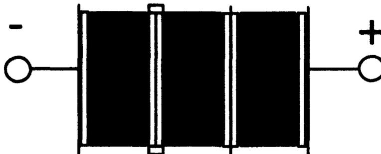
Figure 18. Stylized bipolar battery with non-uniform leakage path.
