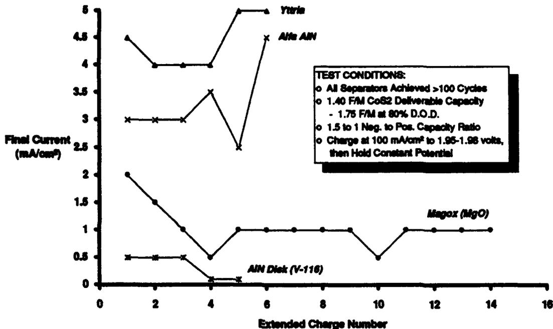
Figure 17. A dimensionally stable aluminum nitride separator achieved the 100 cycle goal with the lowest final currents measured to date.
