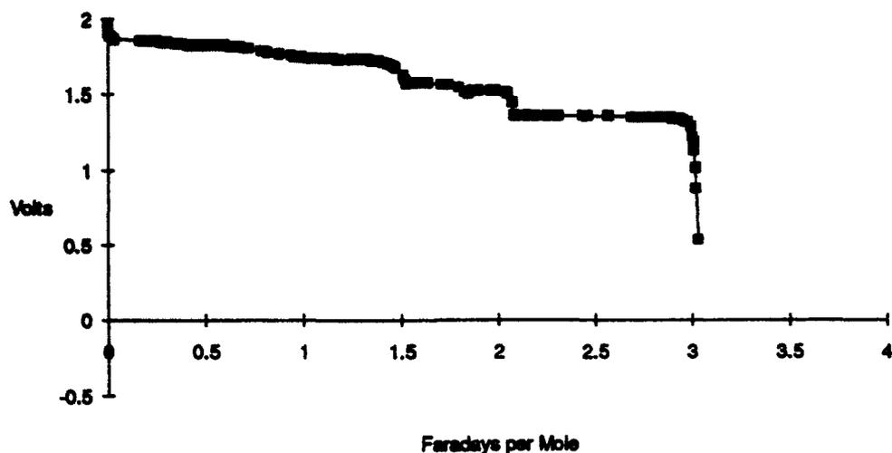
Figure 1. Nickel Disulfide Low Rate Discharge - Cell 2011 Cycle 32, J = 29 mA/sq.cm.
