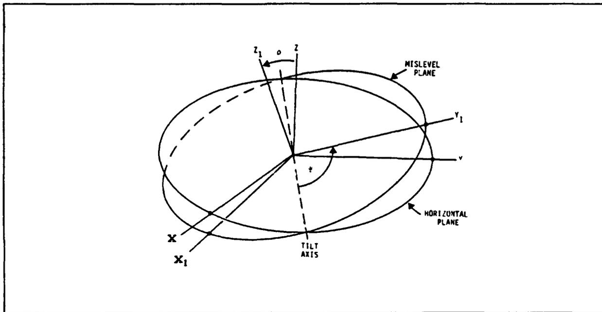
Figure 4-1. Mislevel geometry.
