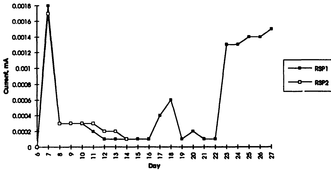
Figure 12. Time-to-Corrosion (RS w. Type 1 PC)
